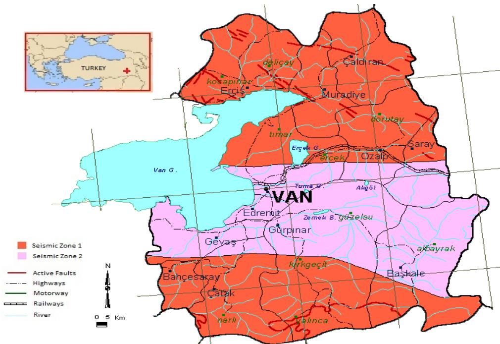
Fig. 2 Seismic Hazard Map of Van Region (where the red areas indicate the first degree zone with a minimum effective acceleration of 0.40 g and the pink areas mark the second degree zone with a minimum acceleration of 0.30 g)
