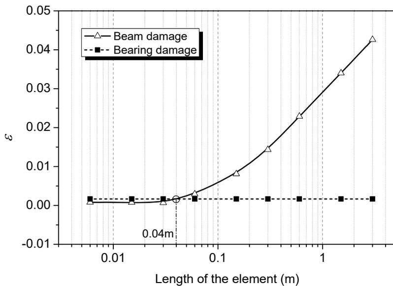
Fig. 9 Comparison between the influence of the bearing damage on the beam vibration mode and that of the bridge beam damage
