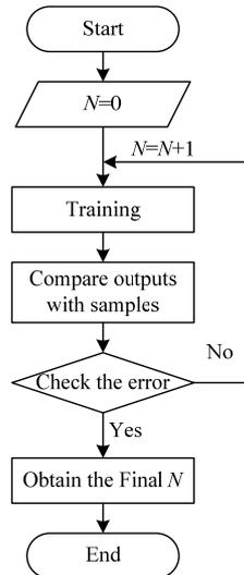
Fig. 2 Determination of the node number in the hidden layer
