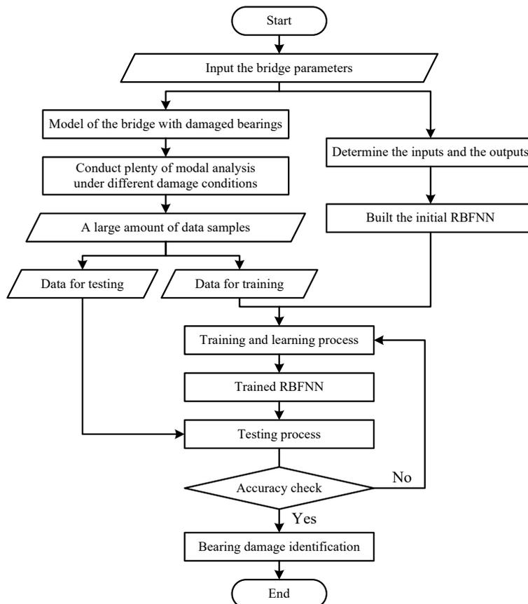
Fig. 3 Bearing damage identification procedure
