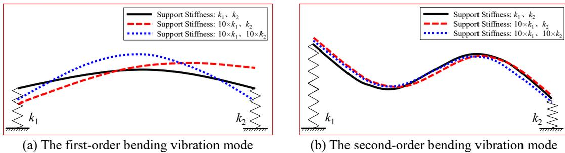
Fig. 6 The influences of the bearing stiffness on beam vibration modes
