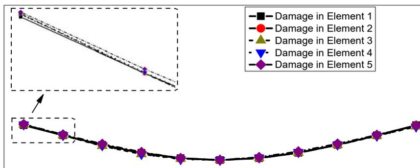
Fig. 8 Influence of the beam damage location on the beam vibration mode
