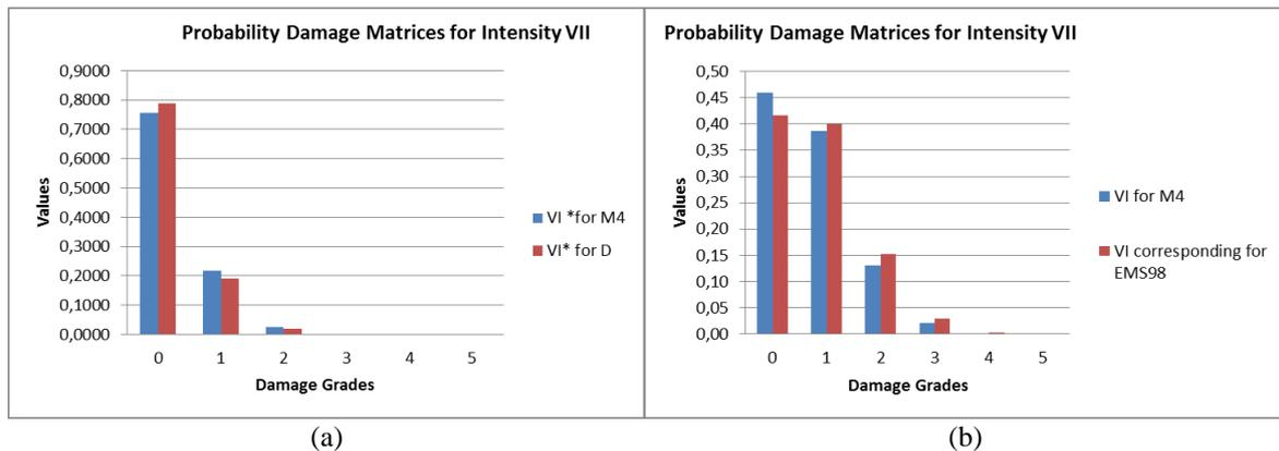
Fig. 10 Damage probability matrices for confined masonry for VII level of earthquake intensity: (a) using typological values ( $V_I^*$ ), (b) using Vulnerability index with added modifiers ( $V_I$ )
