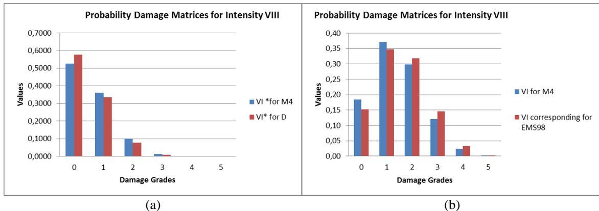
Fig. 11 Damage probability matrices for confined masonry for VIII level of earthquake intensity: (a) using typological values ( $V_I^*$ ), (b) using Vulnerability index with added modifiers ( $V_I$ )
