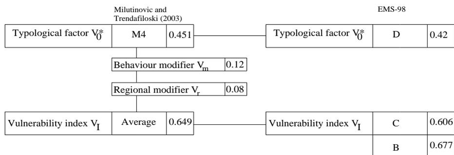
Fig. 8 Applied modifiers factors and corresponding vulnerability classes according to EMS-98
