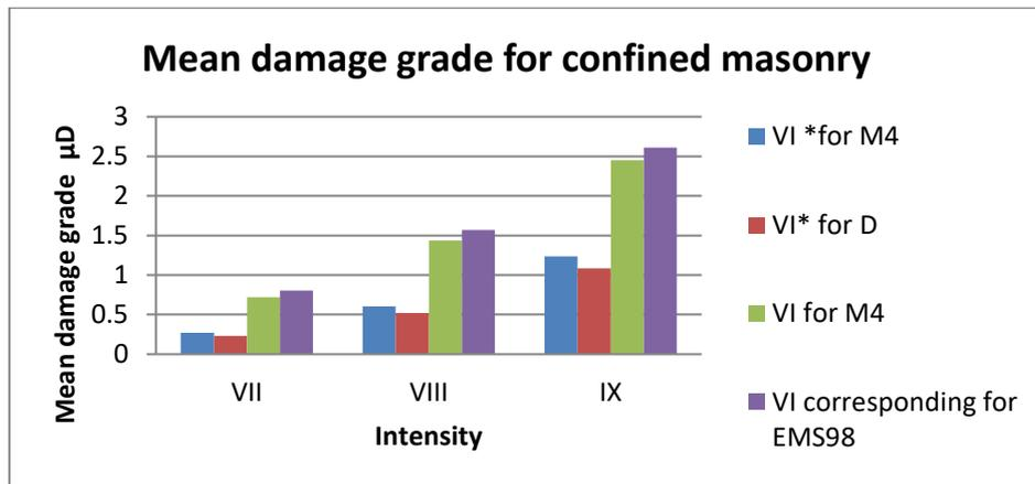
Fig. 9 Mean damage grade calculated for confined masonry buildings
