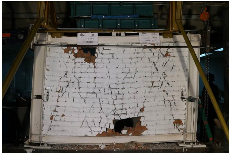
Fig. 10 Failure mode of specimen M-RC-VL
