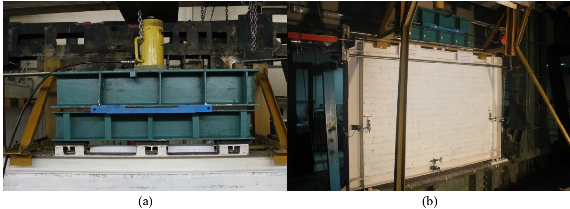
Fig. 2 Setup details; (a) vertical loading and out of plane bracing configuration; (b) out of plane bracing view
