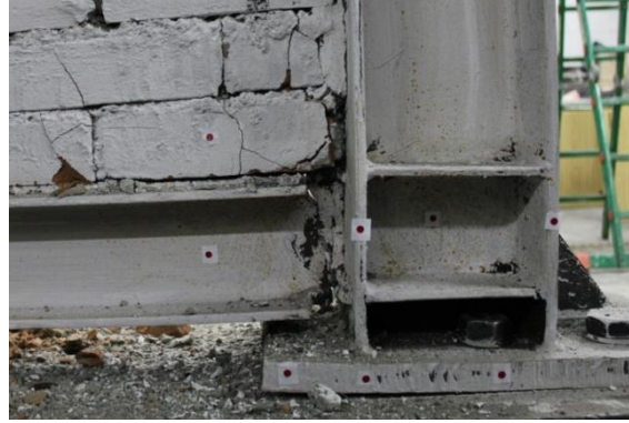
Fig. 15 Failure of pinned connection in specimen M-PC-VL
