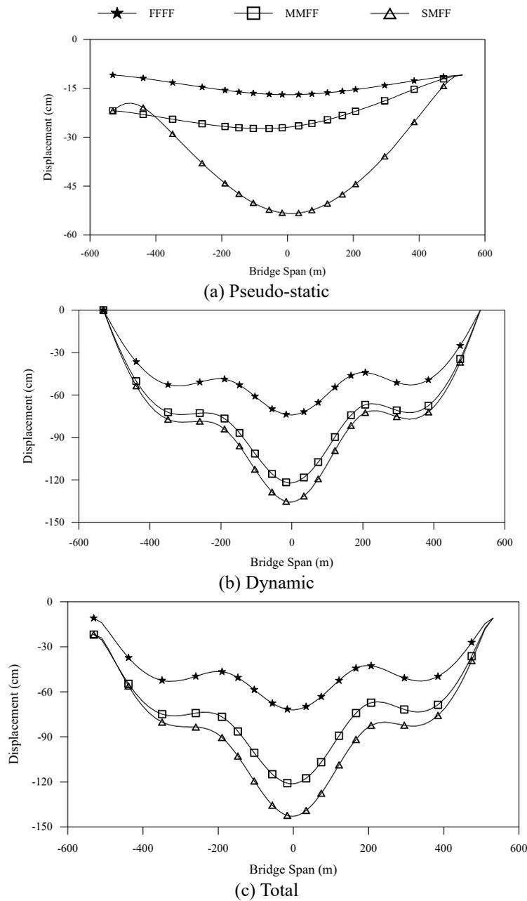
Fig. 4 Mean of maximum vertical displacements of the deck for general excitation case
