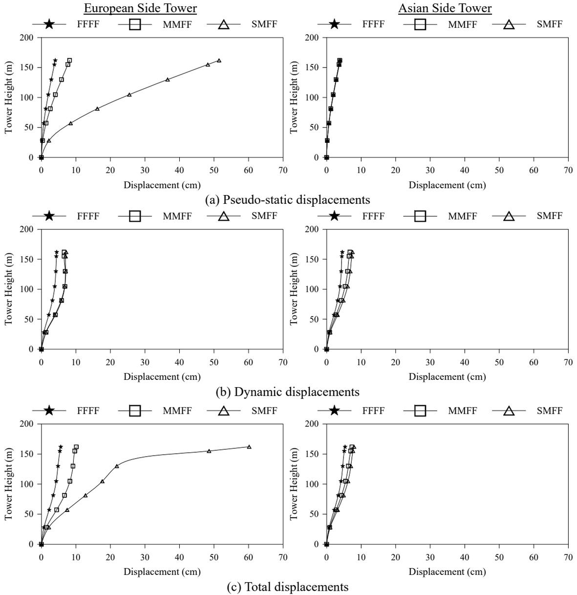
Fig. 5 Mean of maximum horizontal displacements for general excitation case
