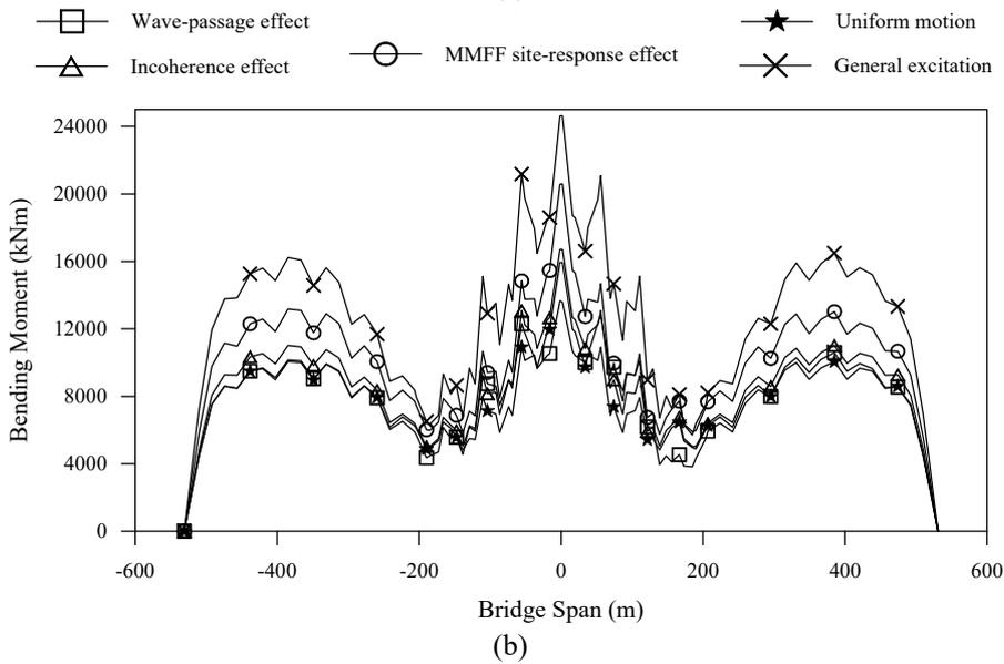
Fig. 9 Mean of maximum total deck (a) displacements and (b) bending moments
