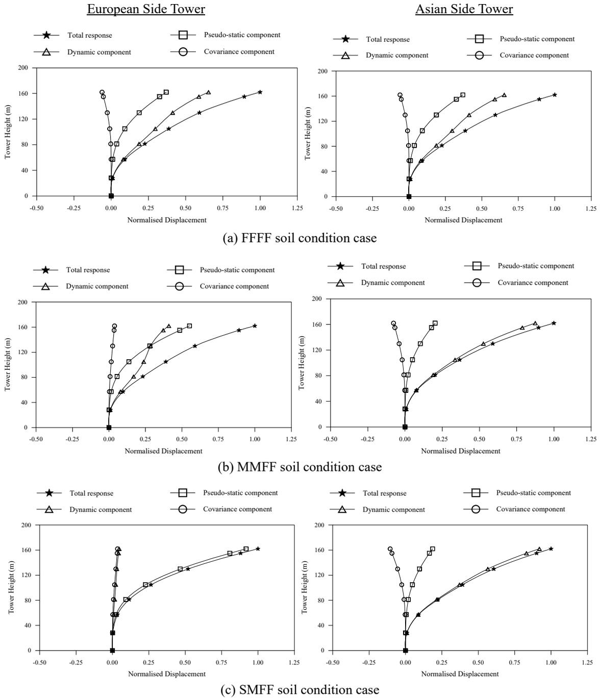
Fig. 8 Normalised displacement variances of two towers for general excitation case
