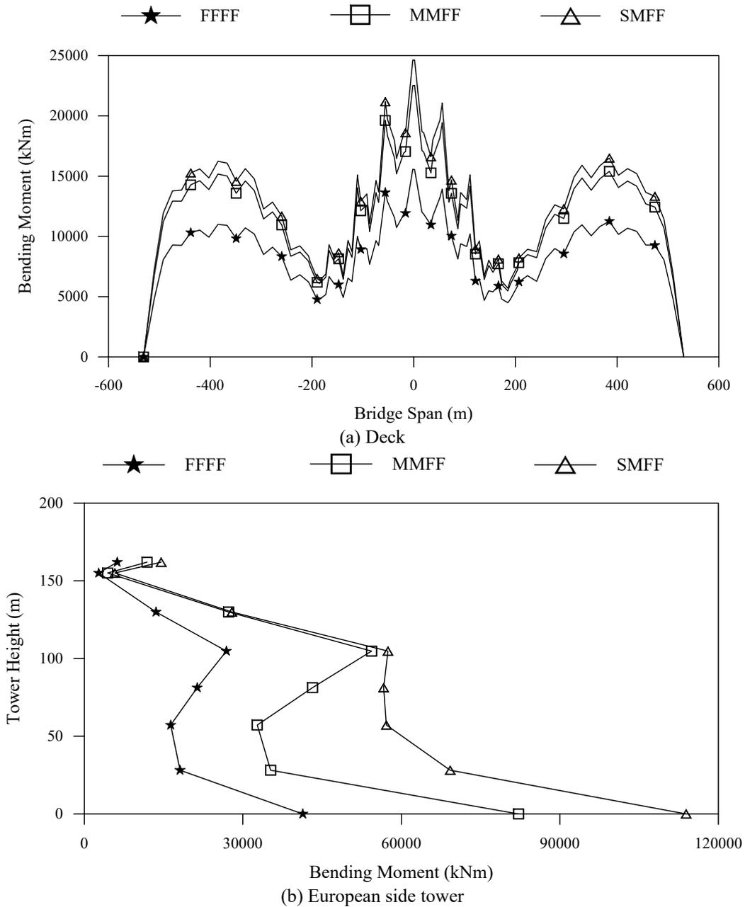
Fig. 6 Mean of maximum total bending moments for general excitation case
