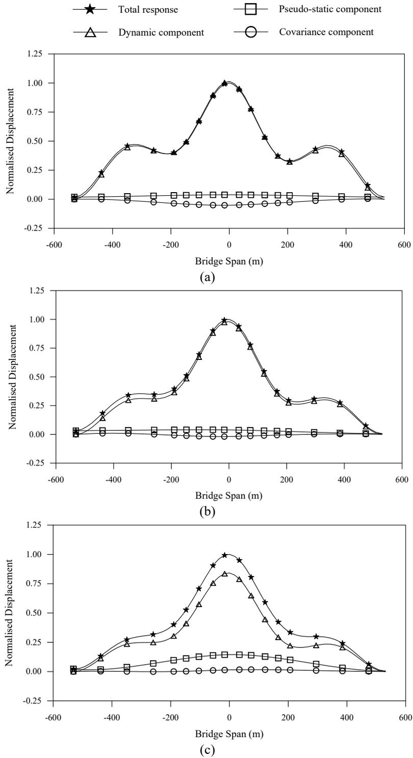
Fig. 7 Normalised displacement variances of the deck for general excitation case (a) FFFF soil condition, (b) MMFF soil condition, and (c) SMFF soil condition
