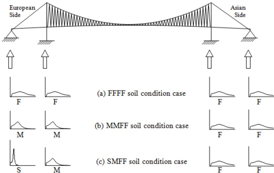
Fig. 3 Suspension bridge subjected to spatially varying ground motions in the vertical direction for the different soil condition case
