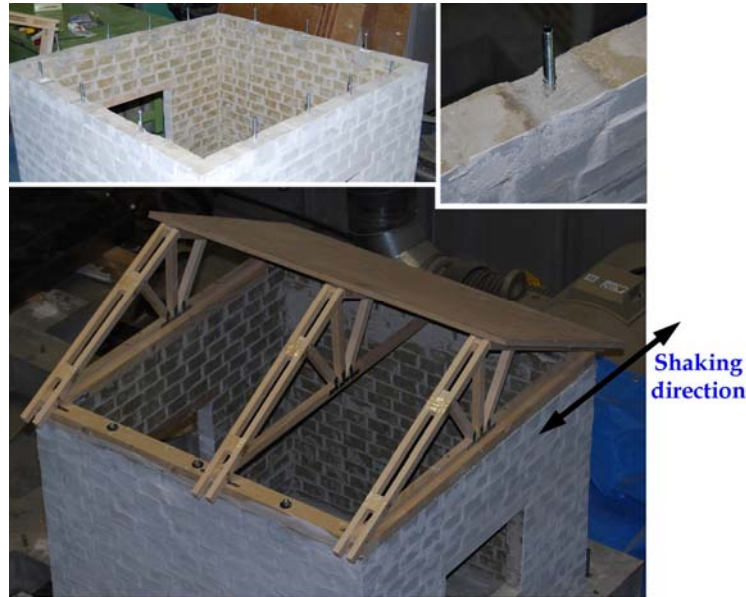
Fig. 4 Wall connection detail of roof to wall
