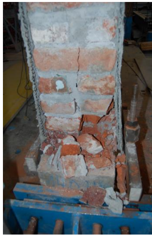
(a) midplane splitting at the bottom corner, specimen W2
