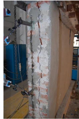
(b) splitting in half of the boundary column, specimen W7
