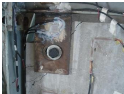
(a) Crack at Left-Top Corner
