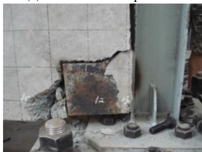
(c) Crushing at Left-Bottom Corner (Back Side)
