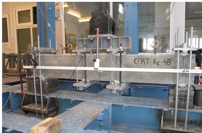
Fig. 6 Experimental set-up for the FRCM strengthened beam under fully reversing cyclic loading
