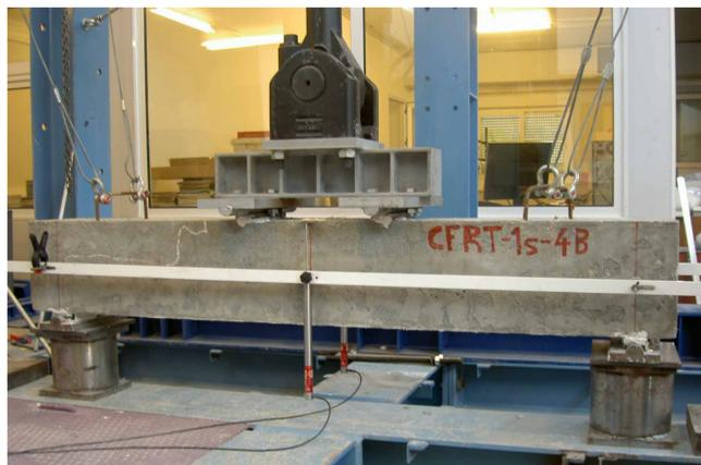
Fig. 5 Instrumentation of the FRCM strengthened beams
