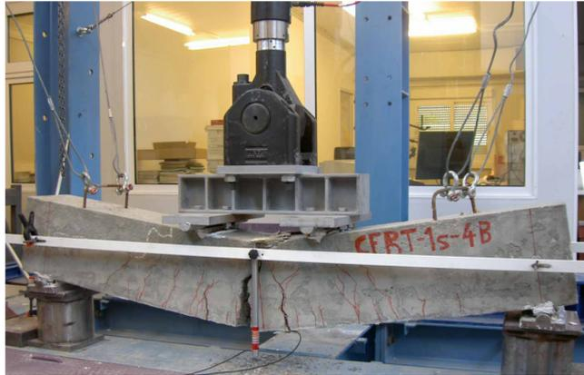
Fig. 21 Failure of the RC beam strengthened with the FRCM jacket (J1), under static monotonic 4-point bending
