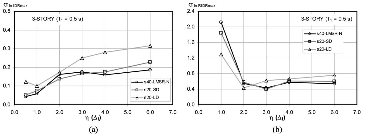
Fig. 12 Effect of the ground motion duration on dispersion of 3-R frame model: (a) dispersion of  $IDR_{max}$  and (b) dispersion of  $RIDR_{max}$
