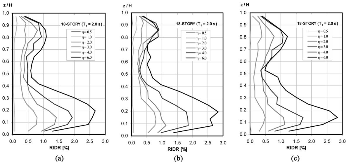
Fig. 9 Height-wise distribution of median  $RIDR$  for 18-R frame model obtained from three suites of ground motions: (a) s40-LMSR-N, (b) s20-SD and (c) s20-LD
