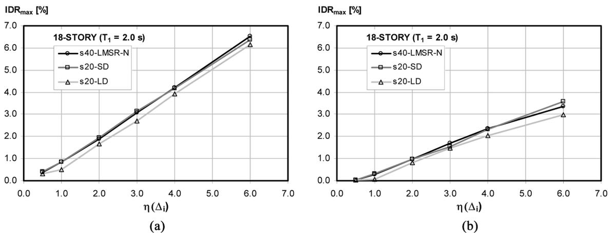
Fig. 13 Effect of ground motion duration on 18-R: (a) median  $IDR_{max}$  and (b) median  $IDR_{max}$
