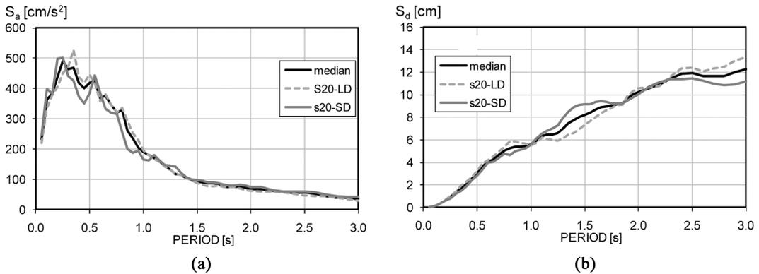
Fig. 2 Comparison of elastic spectra corresponding to the set of motions under consideration: (a) acceleration, (b) displacement
