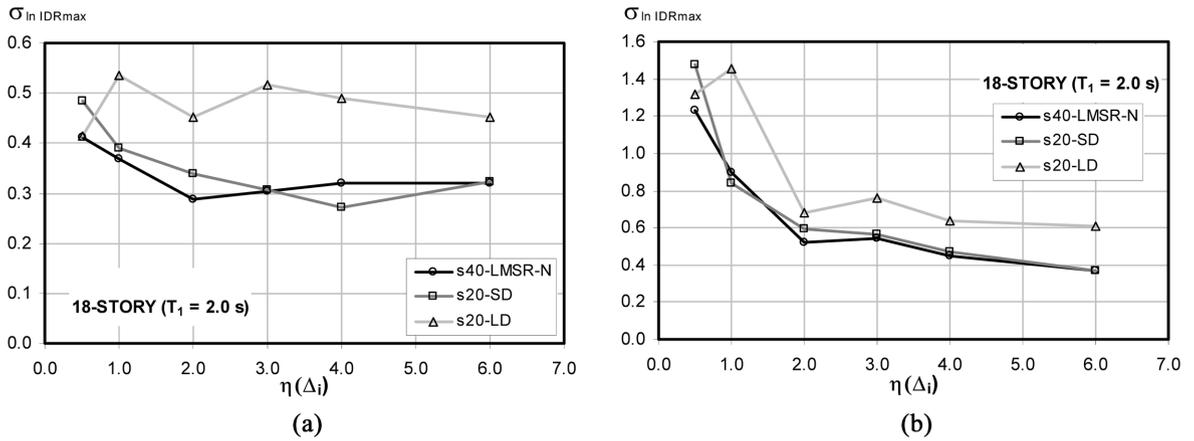
Fig. 14 Effect of the ground motion duration on dispersion of 18-R frame model: (a) dispersion of  $IDR_{max}$  and (b) dispersion of  $RIDR_{max}$
