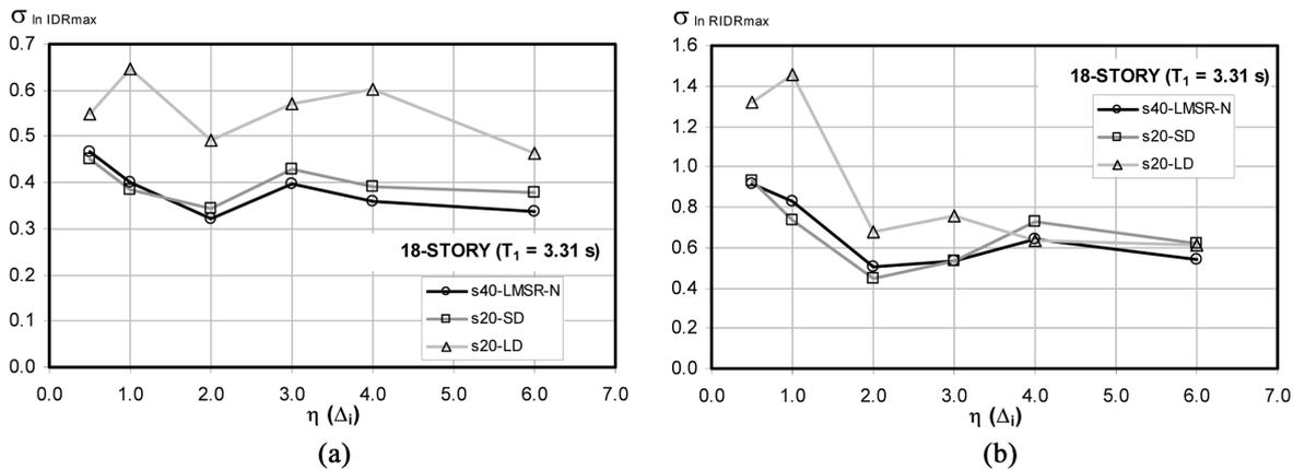
Fig. 16 Effect of the ground motion duration on dispersion of 18-F frame model: (a) dispersion of  $IDR_{max}$  and (b) dispersion of  $RIDR_{max}$
