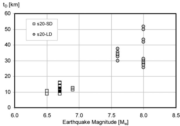
Fig. 3 Distribution of strong motion duration and earthquake magnitude for the sets s20-SD and s20-LD used in this investigation
