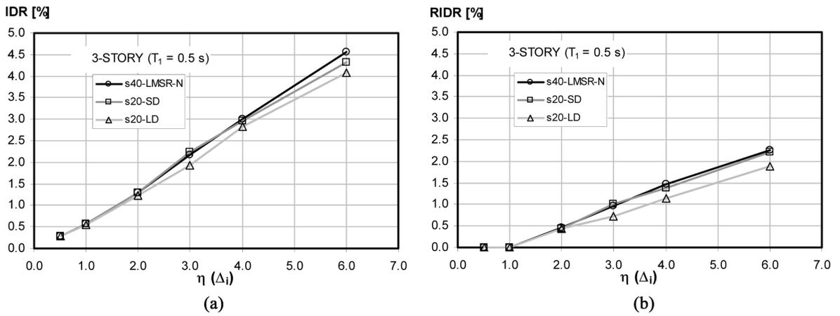
Fig. 11 Effect of ground motion duration on 3-R frame model: (a) median  $IDR_{max}$  and (b) median  $RIDR_{max}$
