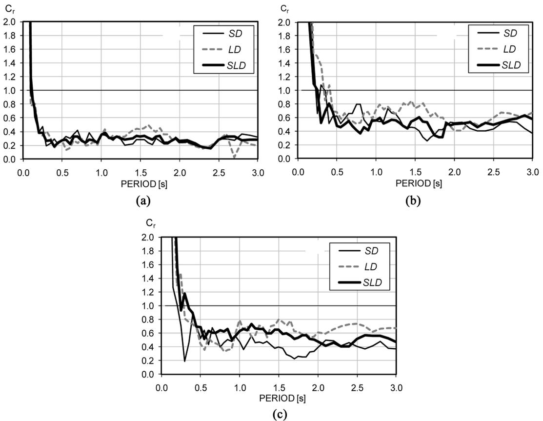
Fig. 4 Effect of strong motion duration on median residual displacement ratios for: (a) R=2, (b) R=4 and (c) R=6
