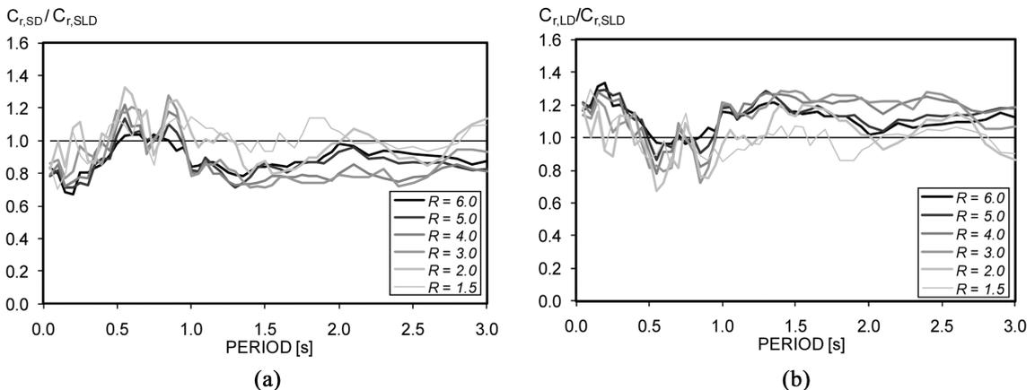
Fig. 6 Mean  $C_r$  computed from each ground motion duration set normalized with respect to mean  $C_r$  from all 40 ground motions: (a) short-duration set and (b) long-duration set
