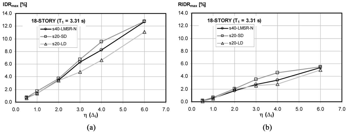
Fig. 15 Effect of ground motion duration on 18-F frame model: (a) median  $IDR_{max}$  and (b) median  $RIDR_{max}$
