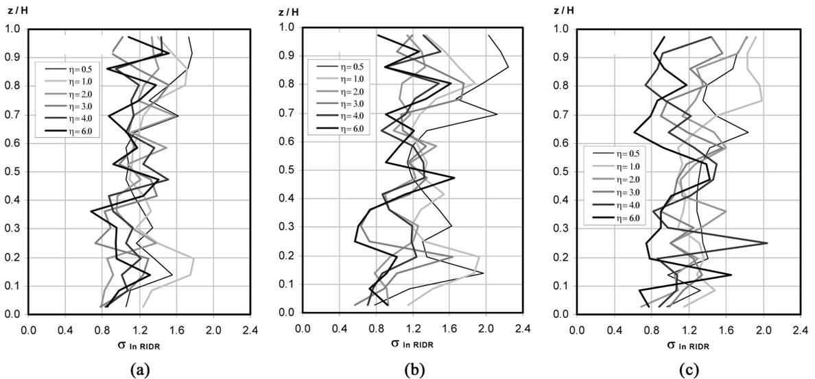
Fig. 10 Height-wise dispersion distribution of  $RIDR$  for 18-R frame model obtained from three suites of ground motions: (a) s40-LMSR-N, (b) s20-SD and (c) s20-LD
