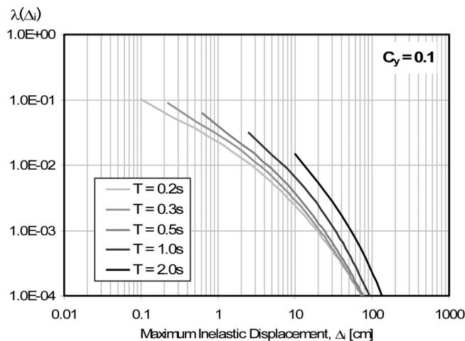
Fig. 8 Maximum inelastic displacement seismic hazard curve corresponding to  $C_y = 0.1$  and five different fundamental periods of vibration (Taken from: Ruiz-García and Miranda 2005)
