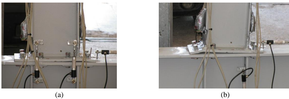
Fig. 14 Deformation of the connection during a cyclic loading
