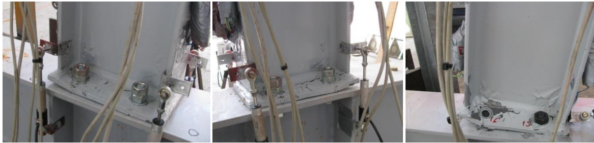
Fig. 13 Deformation of connection elements during experimental testing
