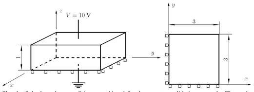
Fig. 1 Sketch of the boundary conditions considered for the actuator validation example. Three planes of symmetry considered in x = y = z = 0; electric potential prescriptions at the top and bottom planes. Measures in mm
