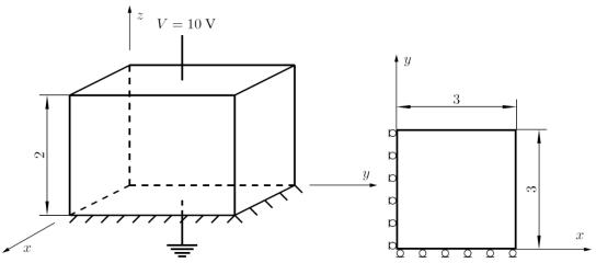
Fig. 4 Sketch of the boundary conditions considered for the third piezoelectric example. Two planes of symmetry considered in x = y = 0; electric potential prescriptions at the top and bottom planes; the latter face clamped. Measures in mm
