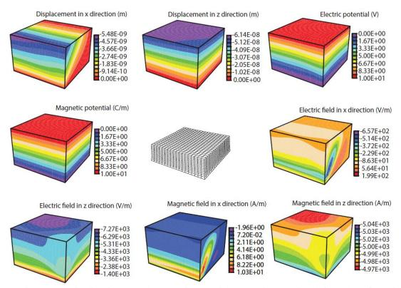
Fig. 6 Displacement in directions x and z, electric potential, magnetic potential, deformed configuration amplified  $10^5$ , electric and magnetic fields in directions x and z distributions for piezo-electro-magnetic clamped case
