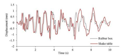
Fig. 5 Comparison of displacements of the rubber box (box 1A, see Fig. 1) and the shake table, subjected to the same highly correlated ground motion associated with the strong rock condition
