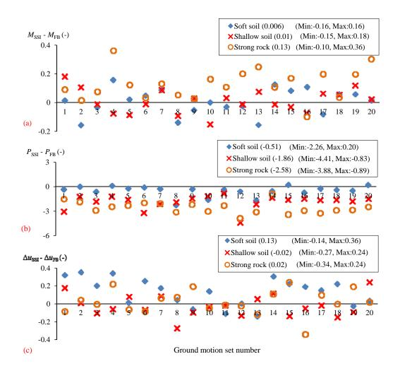
Fig. 11 Consequence of SSI and excitation soil conditions for the maximum values of the normalised (a) bending moment of pier 2A, (b) pounding force, and (c) relative opening displacement between segments 2 and 3
