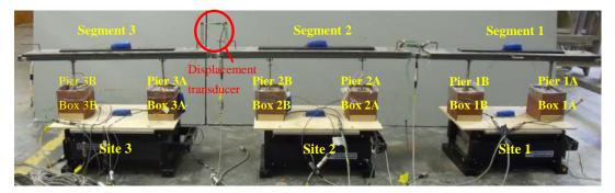
Fig. 1 Setup of the test system with rubber sandboxes
