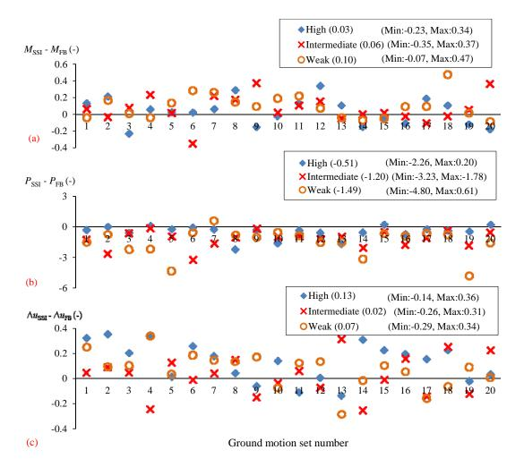
Fig. 12 Consequence of SSI and coherency loss for the maximum values of the normalised (a) bending moment of pier 3A, (b) pounding force, and (c) relative opening displacement between segments 2 and 3
