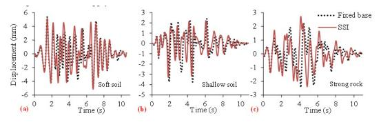
Fig. 6 Absolute displacements of segment 1, with and without SSI, for ground motions of (a) soft soil, (b) shallow soil, and (c) strong rock conditions
