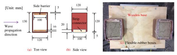
Fig. 4 Flexible rubber boxes: (a) Top view, (b) side view, and (c) top view of boxes filled with sand
