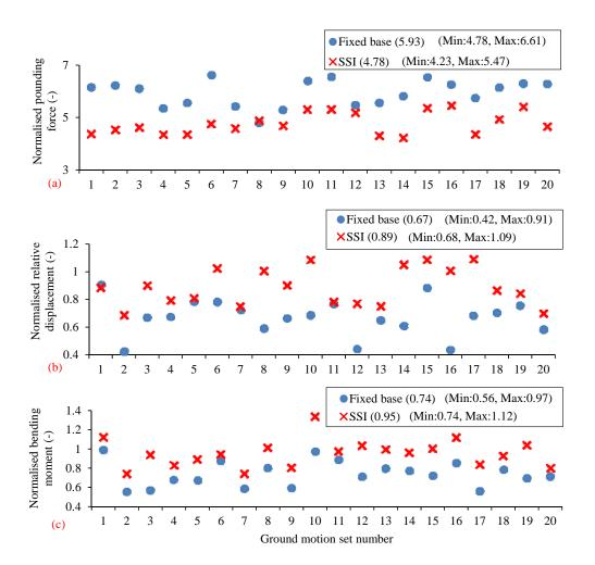
Fig. 10 Consequences of SSI under highly correlated excitations of the shallow soil condition. Maximum values of the normalised (a) pounding force, (b) relative opening displacement between segments 1 and 2, and (c) bending moment of pier 1B
