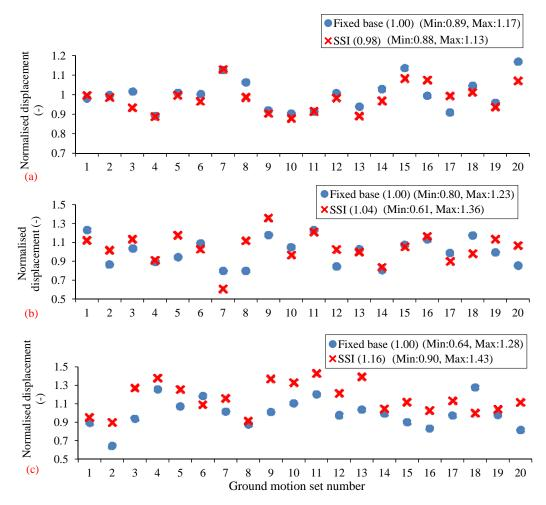
Fig. 7 Consequences of SSI for the normalised maximum absolute displacements of segment 1, without pounding, due to the ground motions of (a) soft soil, (b) shallow soil, and (c) strong rock conditions
