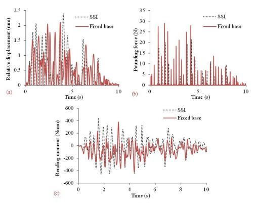
Fig. 9 Consequence of SSI for (a) relative opening displacement, (b) pounding forces of segments 1 and 2, and (c) bending moment of pier 1B, due to highly correlated excitation of shallow soil condition
