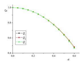
Fig. 2 Variations of the "reference" and approximate values of the normalized axial load Q with a
