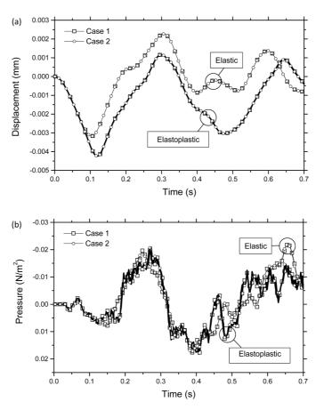
Fig. 8 Time history results considering linear and non-linear material behaviour: (a) vertical displacements at point A and (b) hydrodynamic pressures at point B
