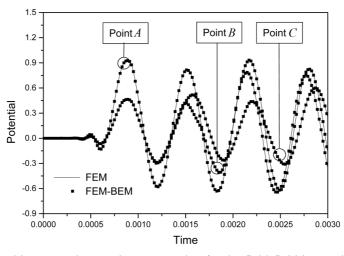
Fig. 2 Time history results at points A, B and C for the fluid-fluid interaction analysis
