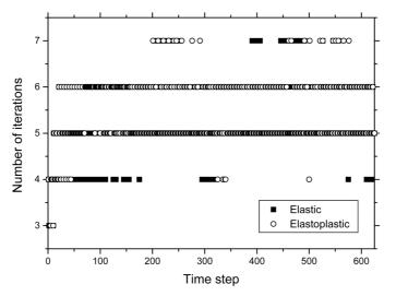
Fig. 5 Number of iterations per time step considering optimal relaxation parameters
