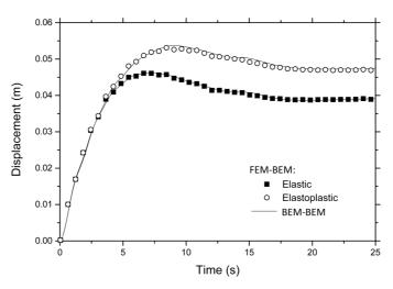
Fig. 4 Horizontal displacements at point A considering elastic and elastoplastic behaviour
