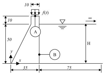
Fig. 7 Dam with a semi-infinite storage-lake: sketch of the model
