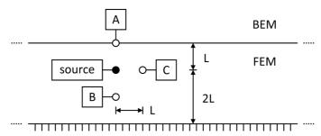
Fig. 1 Sketch of the model for the fluid-fluid interaction analysis
