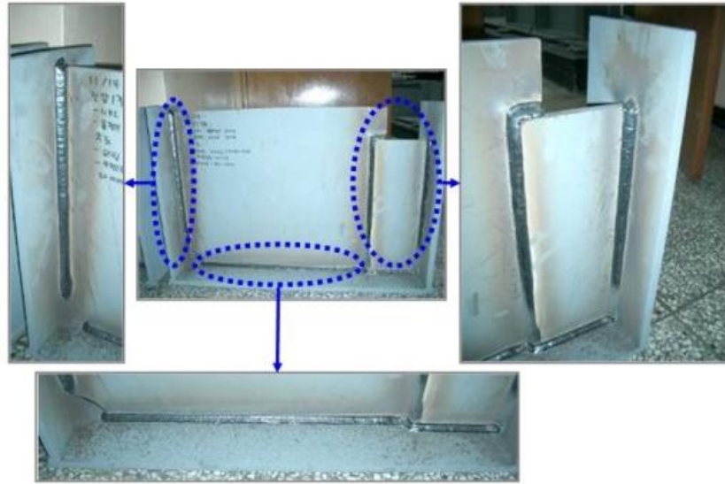
Figure 15. Welding results of the welding test for the mobile welding robot (Voltage: 26V, Current: 250A).
