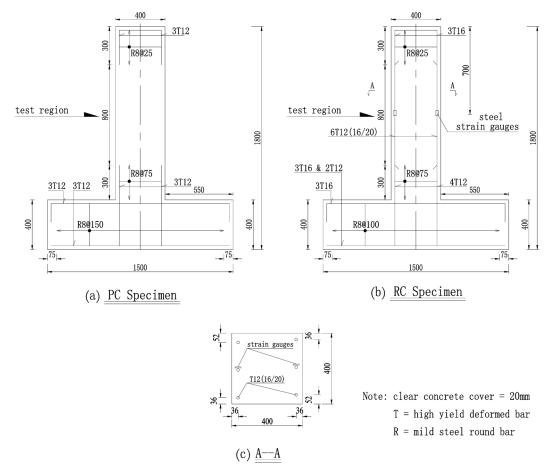
Fig. 2 Details of steel reinforcement
