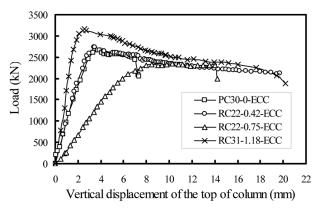
Fig. 8 Load-displacement curves of concrete of eccentrically loaded specimens
