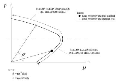
Fig. 3 Failure modes in column interaction diagram
