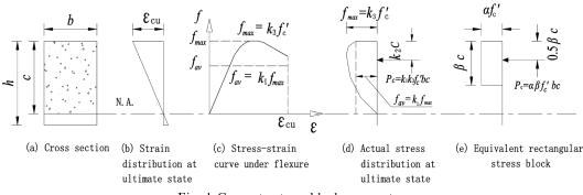
Fig. 1 Concrete stress block parameters
