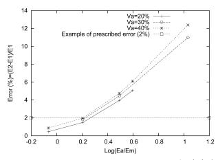
Fig. 7 Evolution of the error between  $E_1$  (analytical model) and  $E_2$  (second ap-proach of the numerical model).  $E_{itz} = 0.5E_m$
