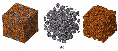
Fig. 2 Finite element models generated for 30% volume fraction of spherical aggre-gates, L = 12 mm, D = 2 mm,  $s_1 = 0.05r$ ,  $s_2 = 0.05r$ : (a) Complete meshed RVE, (b) Meshed aggregates, (c) Meshed matrix
