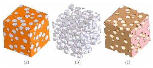
Fig. 1 Unit cell model generated (RVE) for 30% volume fraction of spherical aggregates, L = 12 mm, D = 2 mm,  $s_1 = 0.05r$ ,  $s_2 = 0.05r$ : (a) Complete unit cell, (b) Aggregates, (c) Matrix
