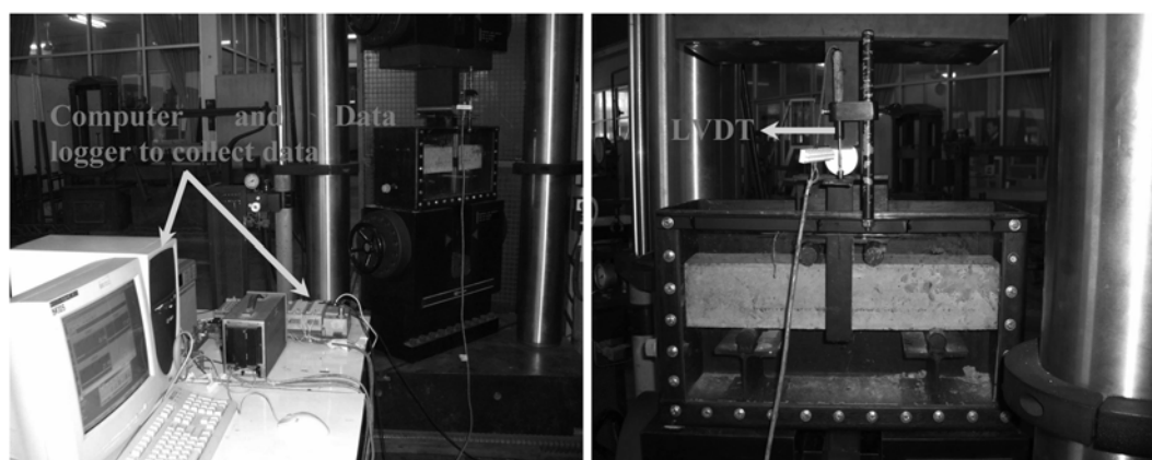
Fig. 2 Set up and equipments used for flexural cyclic loading test
