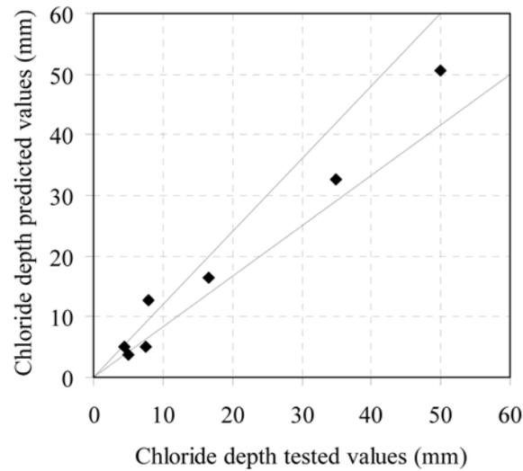
Fig. 5 Relationship between experimental and predicted values of chloride depth
