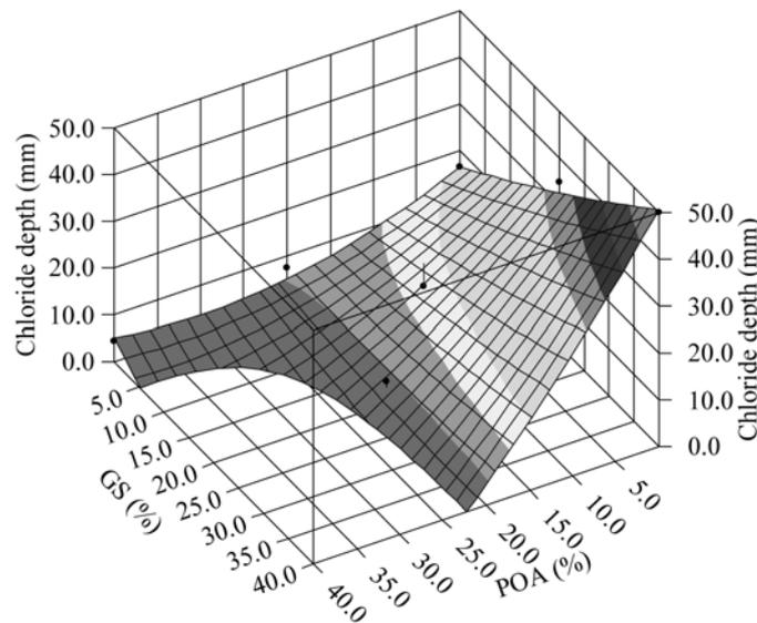
Fig. 6 Isoresponse curve for chloride depth (mm) of mortars
