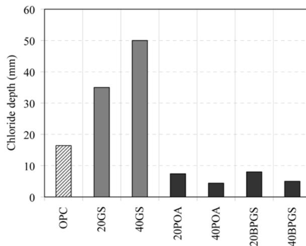
Fig. 4 Chloride depths after 30 days immersion in 3% NaCl (IMT)
