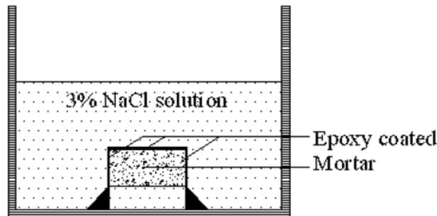
Fig. 2 Immersion of mortar specimen in 3% NaCl solution
