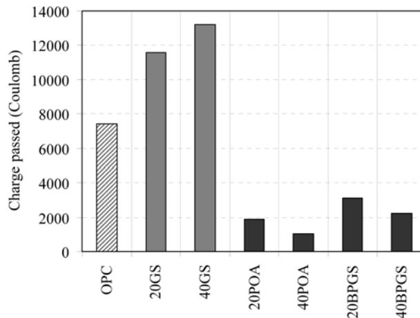
Fig. 3 Charges passed of rapid chloride penetration test (RCPT)
