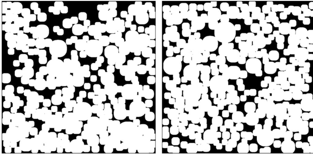
Fig. 9. Simulated 2D pore structure in the hydrated cements (fresh states shown in Fig. 7). Solid phase is indicated in white and pores in black.
