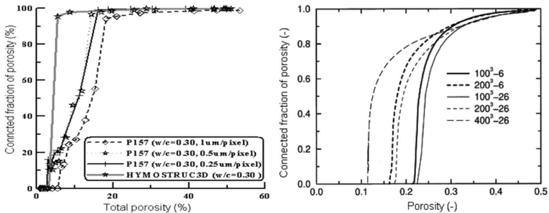
Fig. 14. Evolution of pore de-percolation during hydration (versus porosity), at the left for model cement pastes of which the fresh states were generated by HYMOSTRUC3D and by SPACE [2], and at the right according to Garboczi and Bentz (2001). Influence of resolution is also depicted ( $100^3$ ,  $200^3$  and  $400^3$  correspond to a resolution of 1, 0.5 and  $0.25 \mu\text{m}/\text{pixel}$ , respectively).
