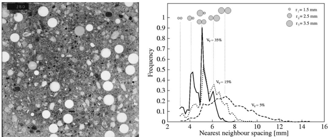
Fig. 2. Section of concrete cube (left) reveals clustering tendency among grains in largest aggregate fraction of 16 mm mono-size ceramic spheres (9.2% by volume) (Stroeven 1973). The nearest neighbor distance distributions for SPACE-generated model ‘concretes’ containing three aggregate grain sizes ( $r$  stands for grain radius) show increasing clustering at higher volume fractions of aggregate (Stroeven and Stroeven 2000).
