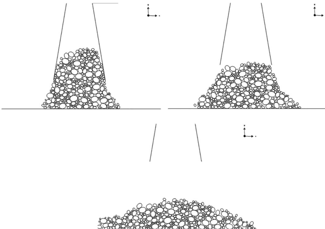
Fig. 12. Stages in the slump test as simulated by HADES
