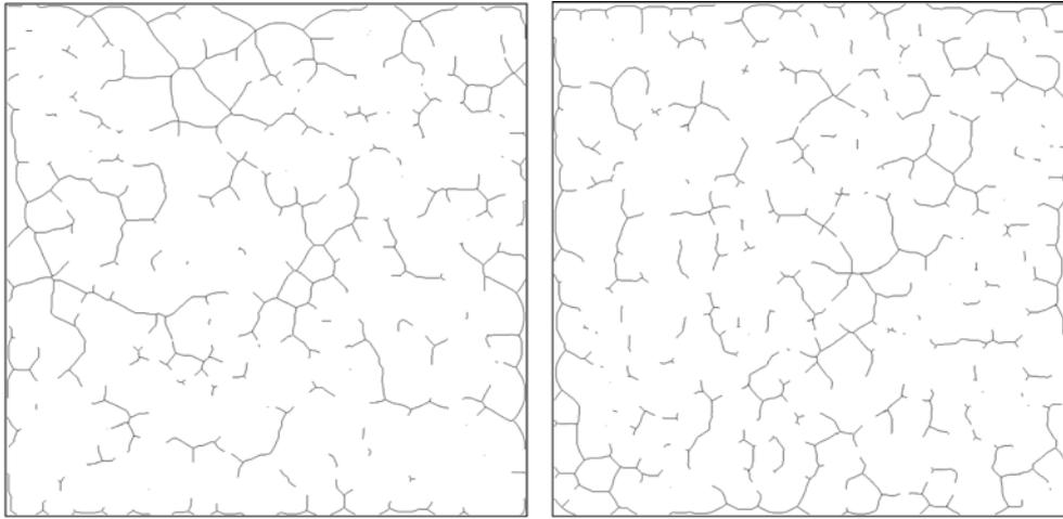
Fig. 11. Skeleton of pore space in 'dynamic' and 'random' packed and hydrated cements (Fig. 7).
