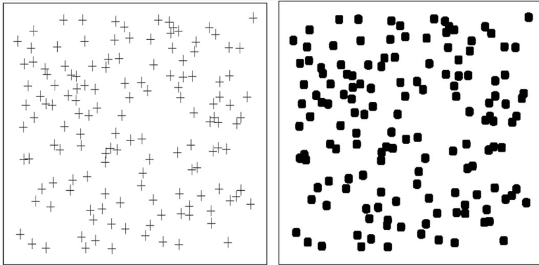
Fig. 1. Random 2-D distribution of points (left) on which mono-size “particles” are positioned with 13% coverage of area whereby overlap is obvious (right).
