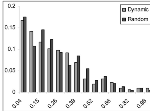
Fig. 8. Probability density of the 2-D surface-to-surface nearest neighbor distance, NND (as bar diagrams) for packing structures generated by concurrent (dynamic) and RSA (random) algorithms as shown in Fig. 7.
