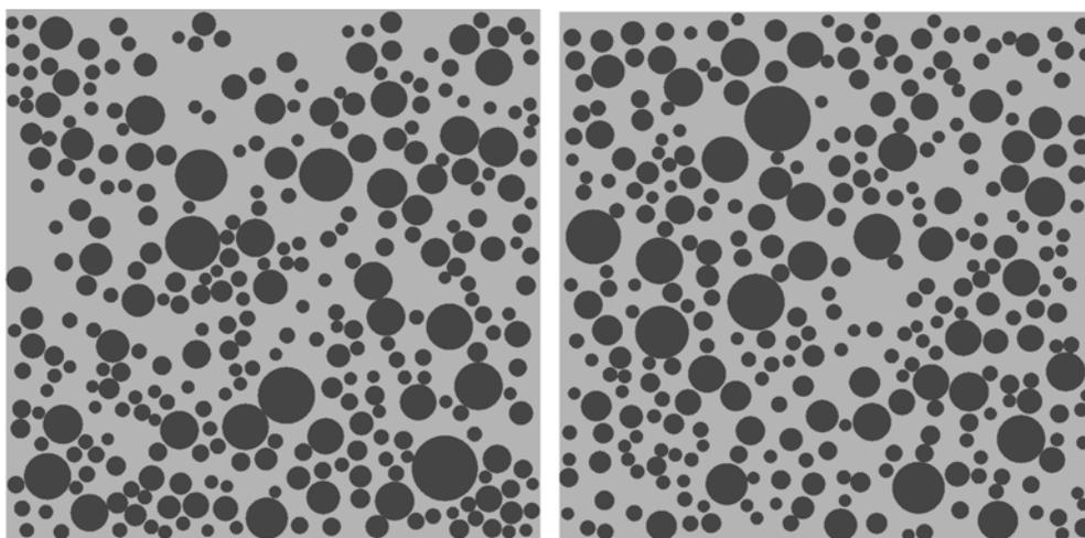
Fig. 7. Two-dimensional “particle” packing patterns simulated by dynamic mixing (left) and by RSA procedure (right) for 40% area coverage. This is employed as the fresh cement paste stage in Fig. 9.
