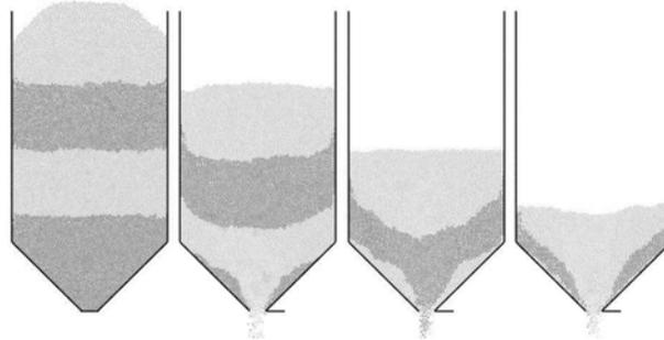
Fig. 4. Silo filled by multi-sized grains during discharge, simulated by HADES. Layers are color-coded to assess discharge mechanisms as a function of mix characteristics (particle size distribution, particle shape) and silo properties (smoothness of internal surfaces, size ratio of particles and opening). For similar type of simulations, see Tüzün and Cleary (2007).
