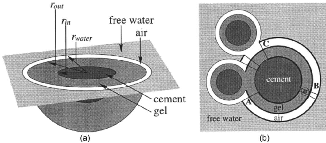
Fig. 6(a) Geometrical representation of hydrated cement and (b) various contact situations between cement particles (according to Stroeven 1999).
