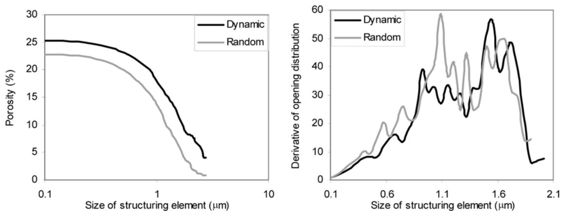
Fig. 10. Cumulative porosity distribution (left) and pore size distribution (right pertaining to Fig. 9
