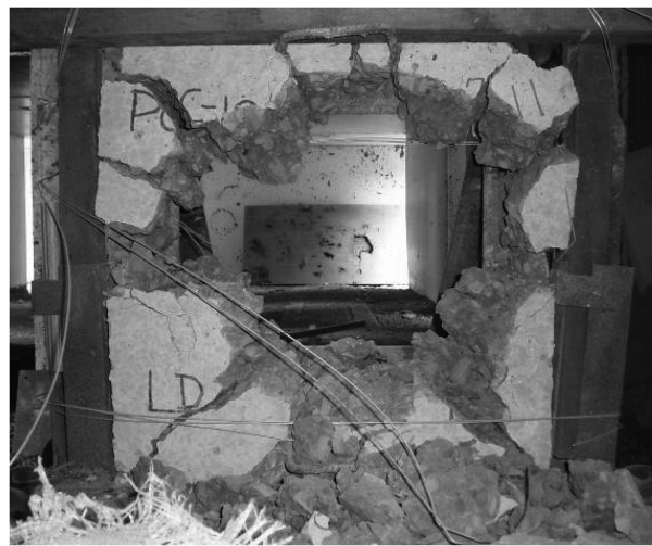
Fig. 8 Failure pattern of plain concrete slabs
