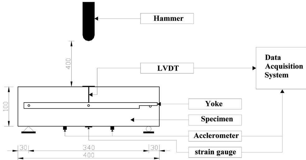
Fig. 1 Schematics of flexural impact test setup
