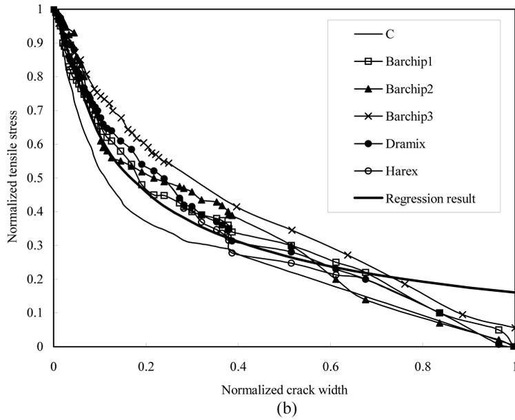
Fig. 3 Normalized axial stress-crack width curves of micro-fiber reinforced concrete in uniaxial tension
