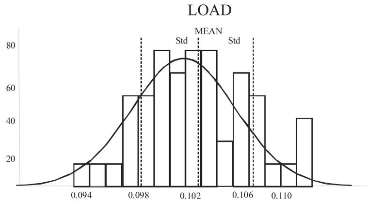
Fig. 11 Histogram and fitted pdf (Weibull) for corbel F25.
