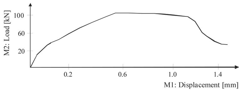
Fig. 7 Load-displacement curve for corbel F25
