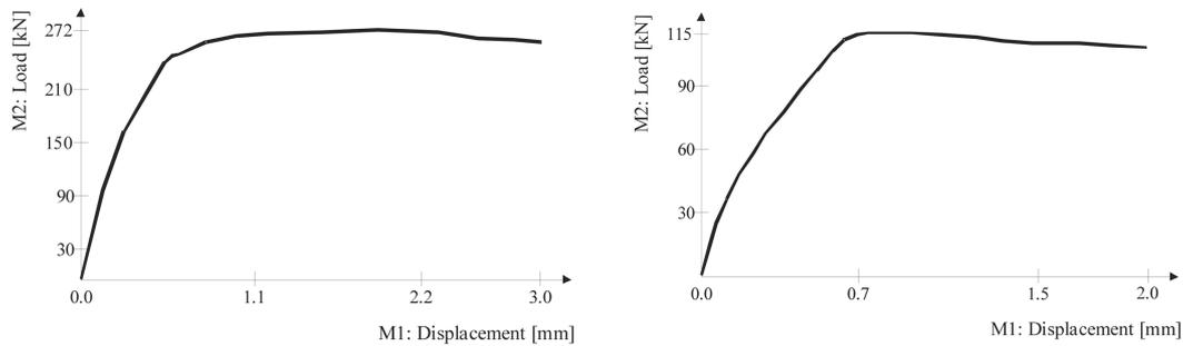
Fig. 17 Load-displacement curve for corbel KR55 (left) and F25 (right)
