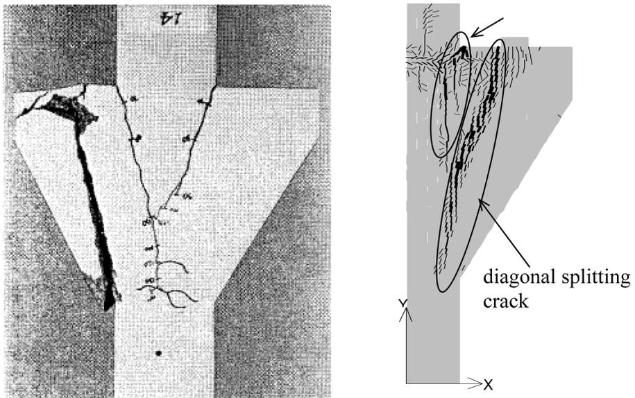
Fig. 8 Experimental and numerical crack patterns for corbel KR14
