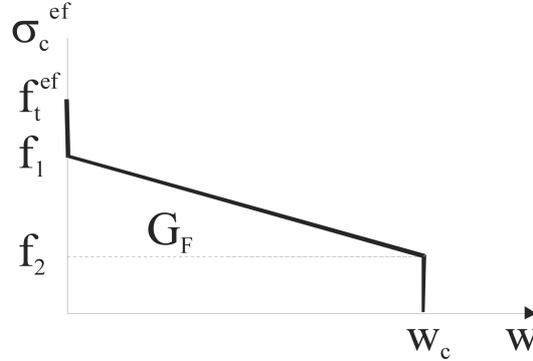
Fig. 2 Crack opening law for SFRC
