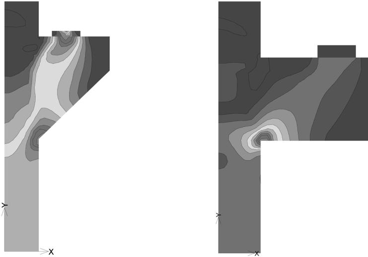
Fig. 5 Modelled compressive principal strain for Kriz-Raths (left) and Fattuhi (right) corbels
