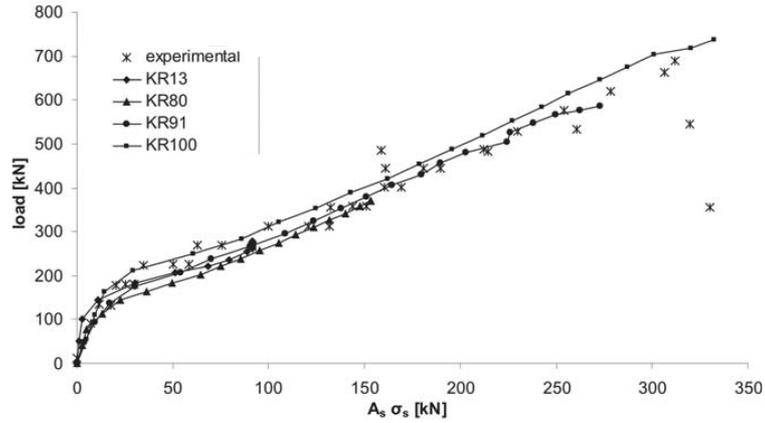
Fig. 4 Load vs. steelstress - numerical to experimental results - Kriz-Raths corbels
