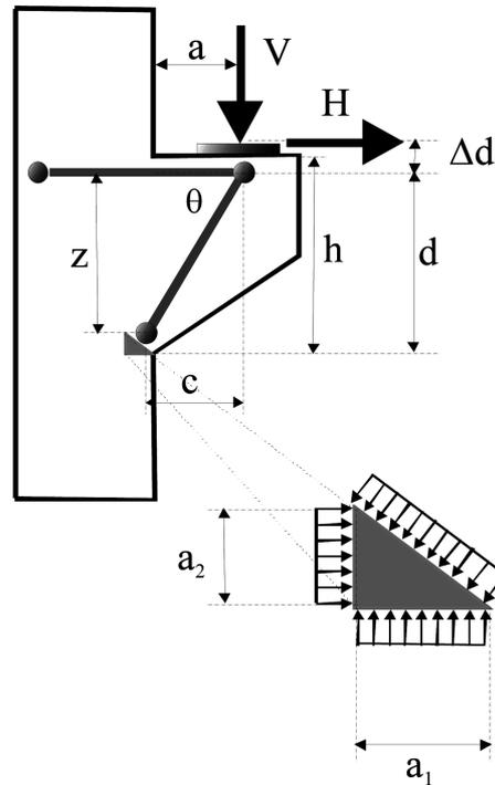
Fig. 1 Corbel sketch with strut-and-tie model
