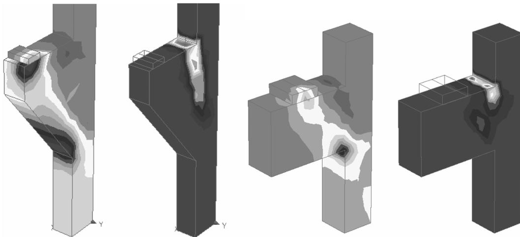
Fig. 18 Min. principal strain and crack width for KR55 (left) and for F25 (right)
