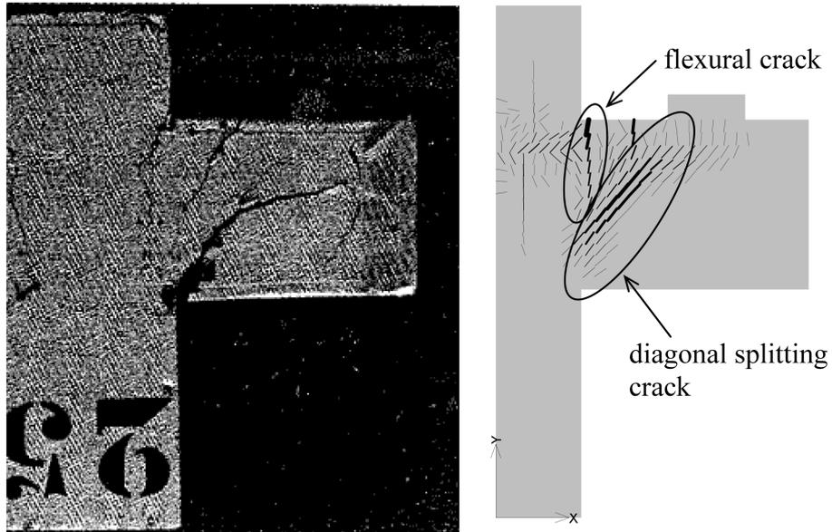
Fig. 9 Experimental and numerical crack patterns for corbel F25
