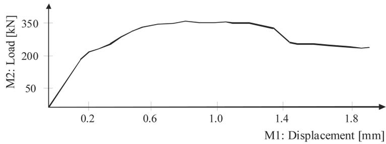
Fig. 6 Load-displacement curve for corbel KR14
