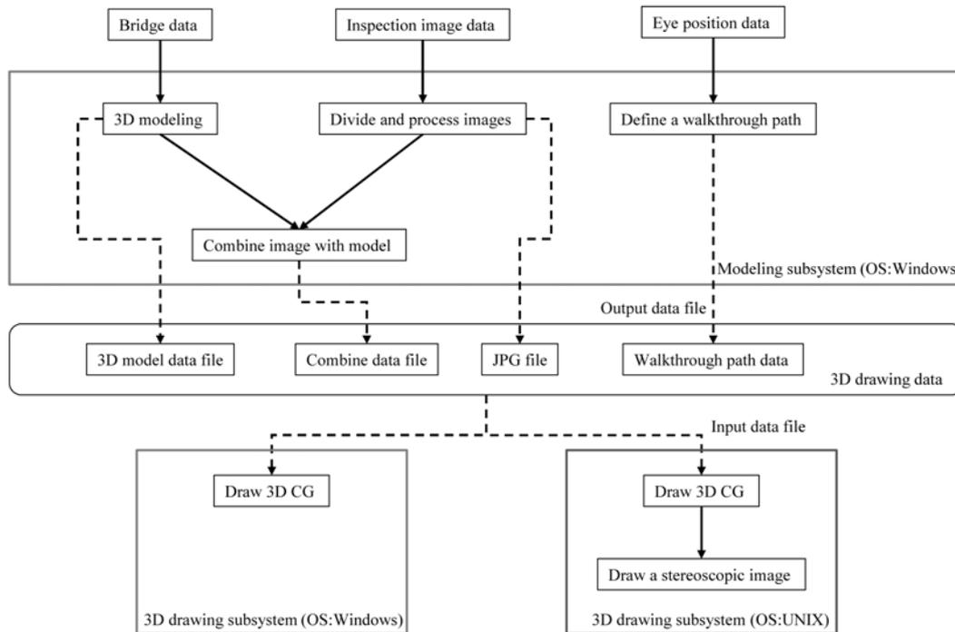
Fig. 1 VR/3DCG system components
