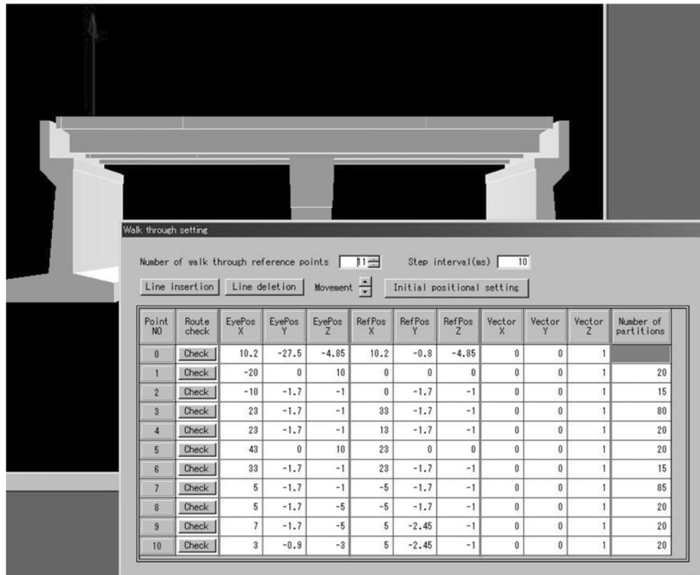
Fig. 4 Sample screen for defining a walkthrough path
