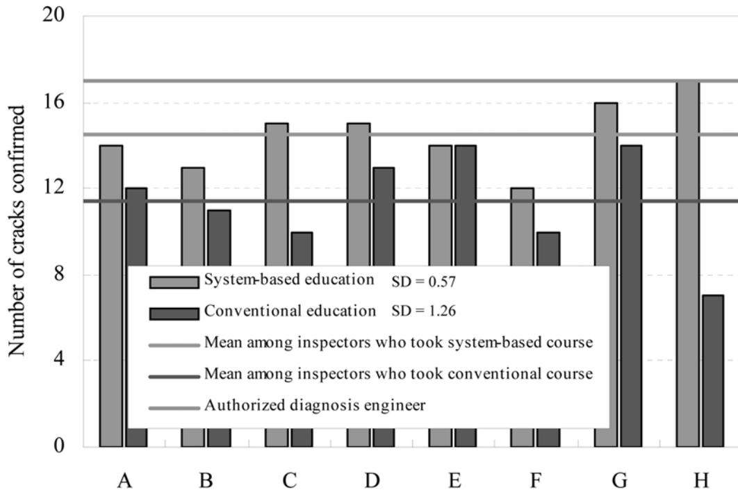
Fig. 8 Verification test results for crack discovery in deck slab
