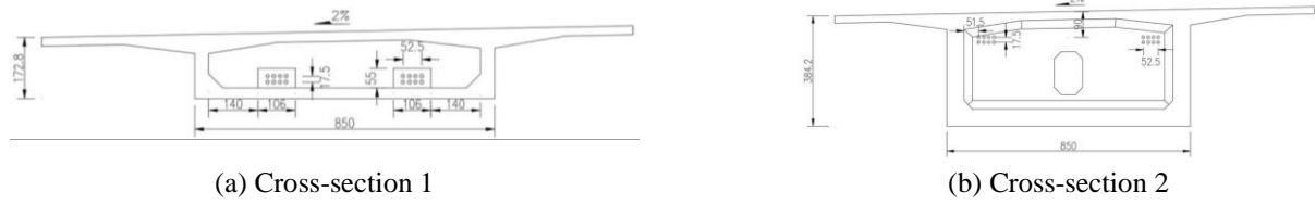
Fig. 12 The critical cross-section details of Hangzhou highway bridge with external prestressing (cm)
