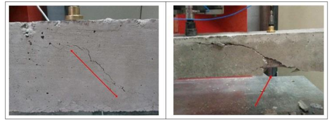
Fig. 7 Crack distribution of CS2 specimen
