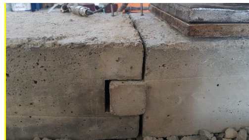
Fig. 11(b) schematic of the keyed joint
