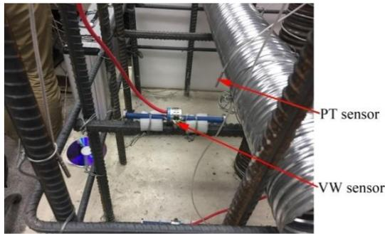
Fig. 7 Sensors tied to the rebars and pipes
