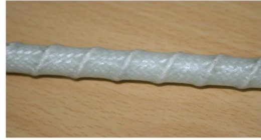
(a) Shape of GFRP rebar
