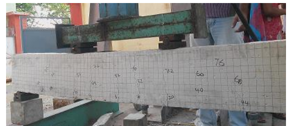
Fig. 7 Crack pattern and failure mode of the reinforced GPC specimen
