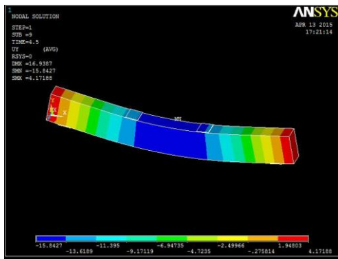
Fig. 13 Typical deflected shape of GPC beam in ANSYS
