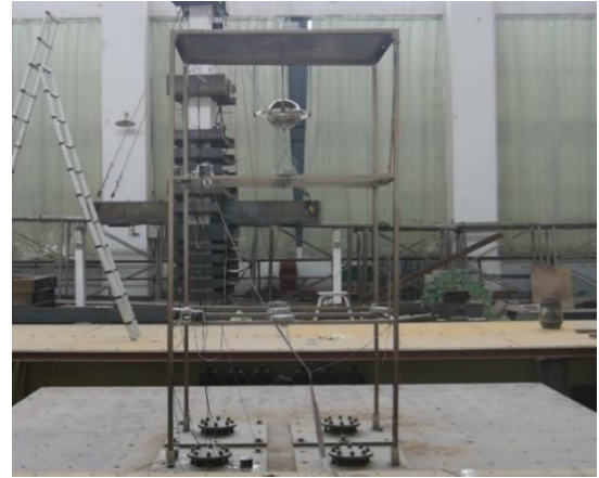
Fig. 4 Shaking table test of the experimental model
