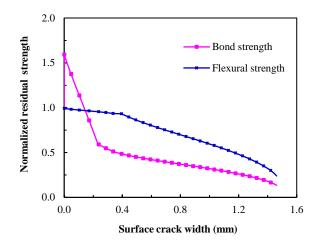
Fig. 6 Normalised residual flexural strength and bond strength versus cover surface crack width
