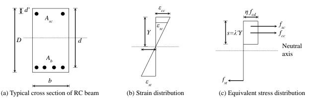
Fig. 2 Flexural analysis of a RC beam section
