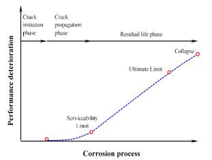
Fig. 1 Schematic representation of performance deterioration of corrosion affected reinforced concrete structures
