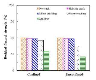
Fig. 9 Normalised residual flexural strength versus cover surface defects for confined and unconfined concrete
