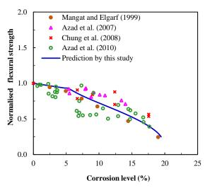
Fig. 5 Normalised residual flexural strength versus corrosion level, compared with available experimental test results
