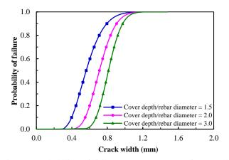
Fig. 11 Probability of failure versus cover surface crack width for various concrete cover depths of confined concrete
