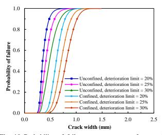
Fig. 10 Probability of failure versus cover surface crack width for various flexural strength deterioration limits of unconfined and confined concrete
