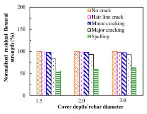
Fig. 8 Normalised residual flexural strength versus cover surface crack defects at different concrete cover depths
