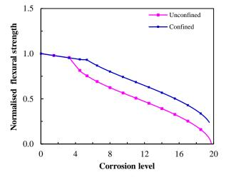
Fig. 7 Normalised residual flexural strength versus corrosion level for confined and unconfined concrete
