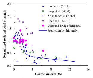
Fig. 3 Normalised residual bond strength versus corrosion level, compared with available field test data of Ullasund Bridge and experimental test results avialeble from various sources
