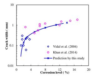
Fig. 4 Equivalent cover surface crack width versus corrosion level, compared with available experimental data from natural corrosion tests in Vidal *et al.* (2004) and Khan *et al.* (2014)
