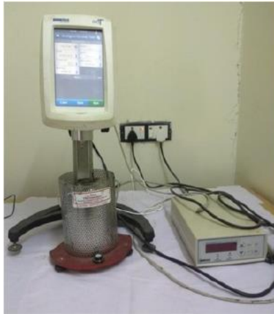
Fig. 1 Brookfield Viscometer DV3T for measuring plastic viscosity of paste
