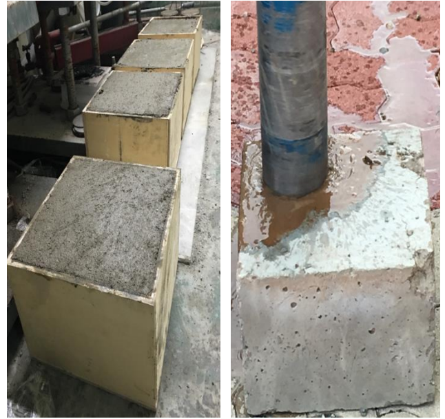
(a) Concrete specimens casted in a mold (b) Coring of damaged specimen
