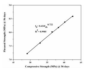
Fig. 12 The Relationship between compressive strength with flexural strength for wet cast PCPB containing crumb rubber at 56 days
