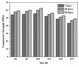
Fig. 4 Compressive strength of wet cast PCPB for different crumb rubber content
