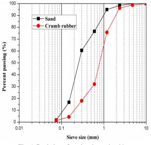
Fig. 1 Gradation of sand and crumb rubber
