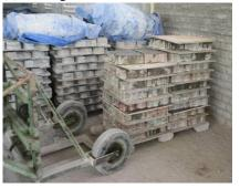
(c) Specimens are arranged for curing
