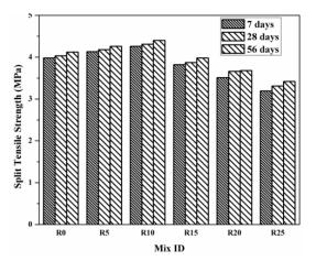
Fig. 5 Split tensile strength of wet cast PCPB for different crumb rubber content
