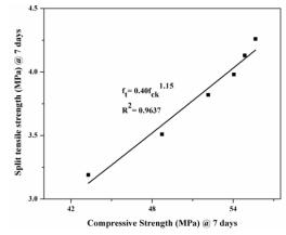
Fig. 7 The relationship between compressive strength with split tensile strength for wet cast PCPB containing crumb rubber at 7 days
