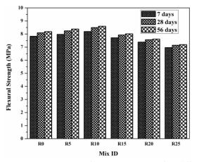
Fig. 6 Flexural strength of wet cast PCPB for different crumb rubber content
