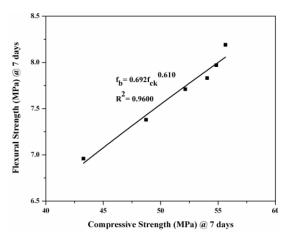
Fig. 8 The Relationship between compressive strength with flexural strength for wet cast PCPB containing crumb rubber at 7 days
