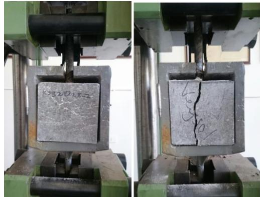
Fig. 4 Pull-out tests of SCMs
