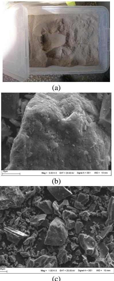
Fig. 2(a) Ground pumice powder (GPP) (b) 10  $\mu\text{m}$  Mag SEM micrographs of GPP (c) 20  $\mu\text{m}$  Mag SEM micrographs of GPP
