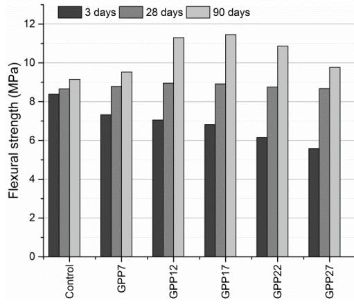
Fig. 9 Flexural tensile strength of SCMs of at the age of 3, 28 and 90-day
