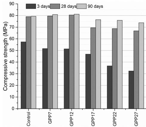
Fig. 8 Compressive strength of SCMs at the age of 3, 28 and 90-day
