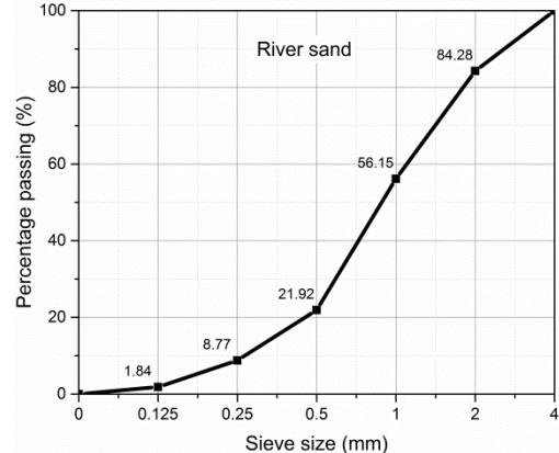
Fig. 3 Particle size distribution of natural river sand
