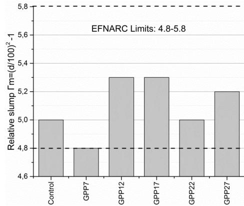
Fig. 5 Relative slump of SCMs
