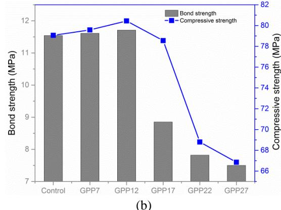
Fig. 12 Variation of bond strengths with respect to compressive strength at the age of 28 d
