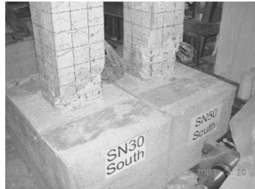
(b) Spalling of cover concrete
