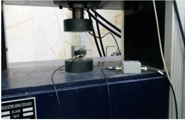
Fig. 5 Servo-electric load frame and AE sensor
