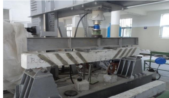
Fig. 7 The arrangement of test set
