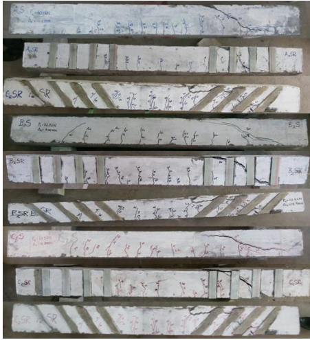
Fig. 15 Crack pattern & failure modes of tested beam
