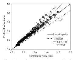
Fig. 12 Comparison between predicted and experimental total deflection for all data points including the data of previous study (Shariq *et al.* 2013)
