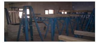
Fig. 3 RC beam specimens under test
