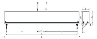
Fig. 1 Details of test specimen (b=100 mm, d=130 mm, D=150 mm, a=750 mm, l=1700 mm, L=1800 mm,  $A_{st}$ =2 $\phi$ 10)
