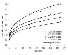
Fig. 9 Comparison between predicted and experimental total deflection for mix group M3
