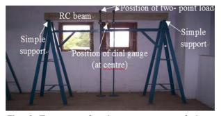
Fig. 2 Test setup for the measurement of timedependent deflection of RC beam
