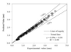
Fig. 11 Comparison between predicted and experimental total deflection for all data points of the present study
