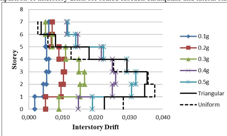
(c) Comparison of interstory drifts for scaled Kobe earthquake and lateral static loads
