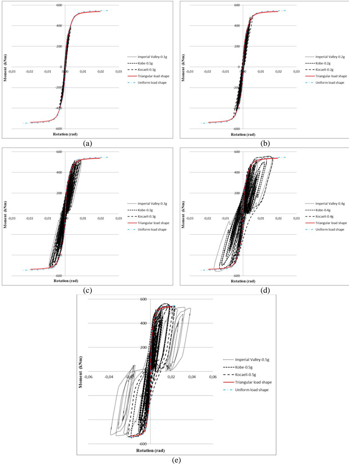
Fig. 10 Moment-rotation curves of lower end of C311a column under nonlinear static and dynamic loads
