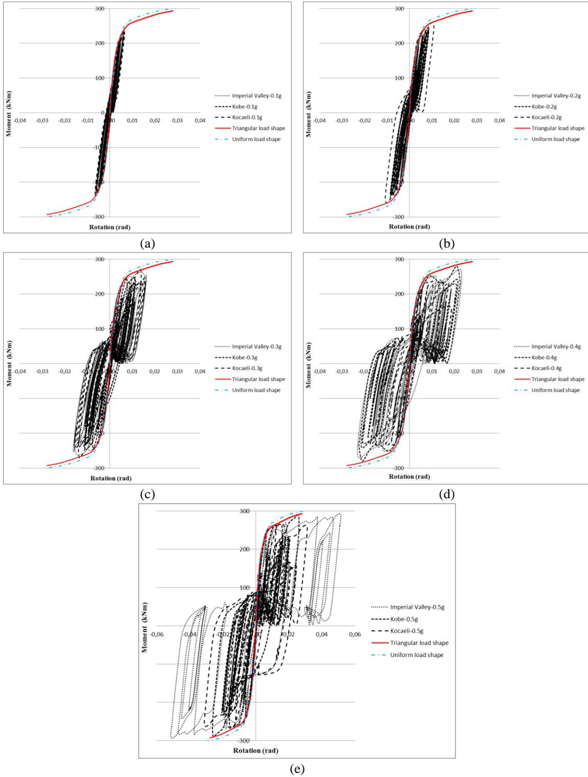
Fig. 12 Moment-rotation curves of left end of B212a beam under nonlinear static and dynamic loads
