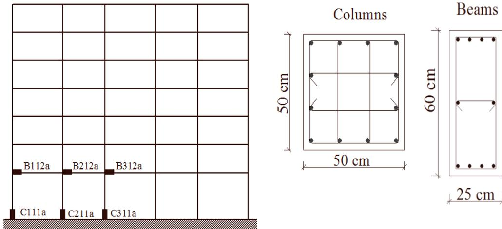
Fig.1 The elevation view of the building and typical element details
