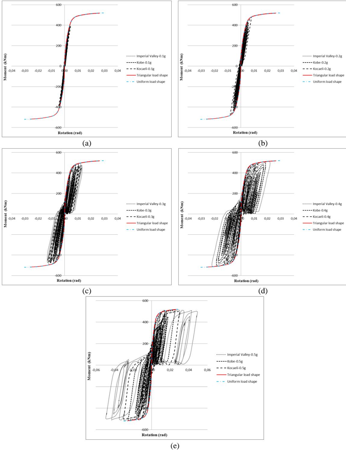
Fig. 8 Moment-rotation curves of lower end of C11a column under nonlinear static and dynamic loads
