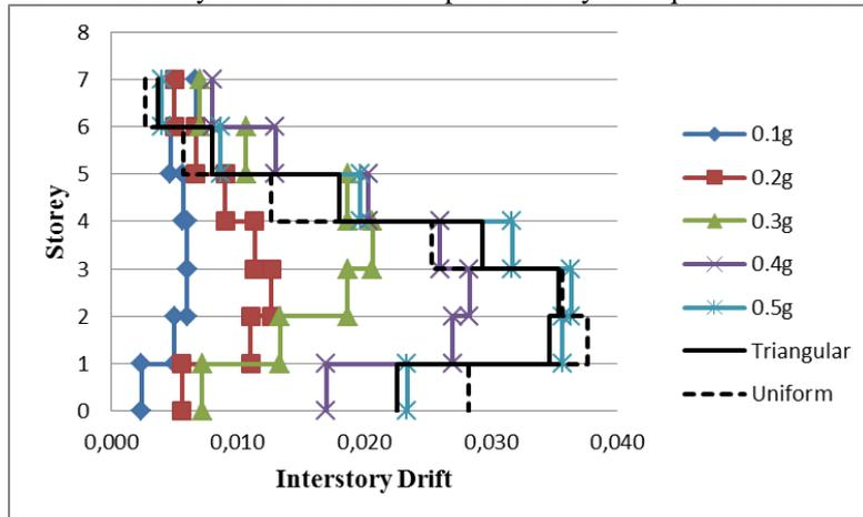
(b) Comparison of interstory drifts for scaled Kocaeli earthquake and lateral static loads
