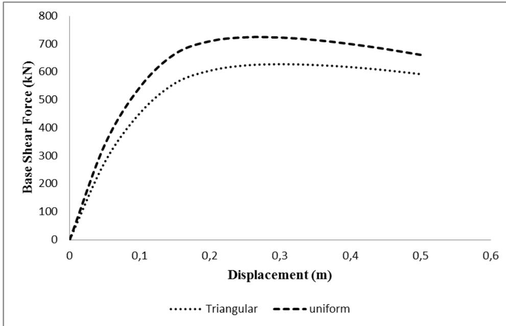
Fig. 5 Capacity curves of the building according to various load shapes
