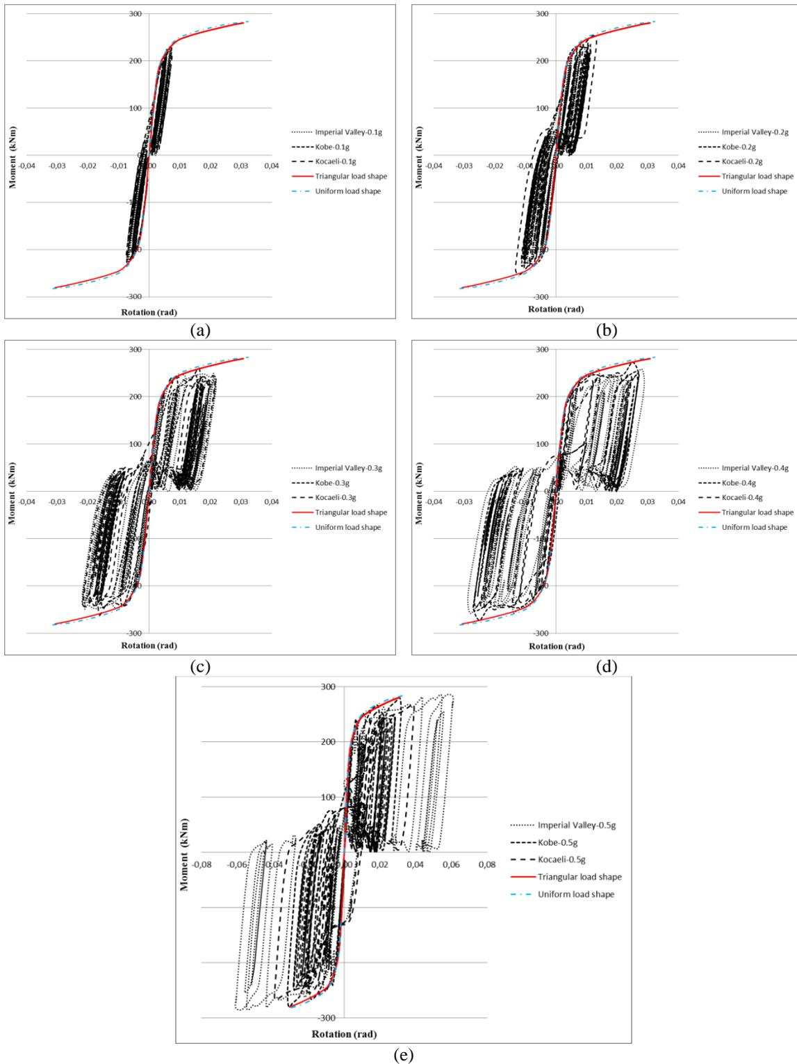
Fig. 11 Moment-rotation curves of left end of B112a beam under nonlinear static and dynamic loads
