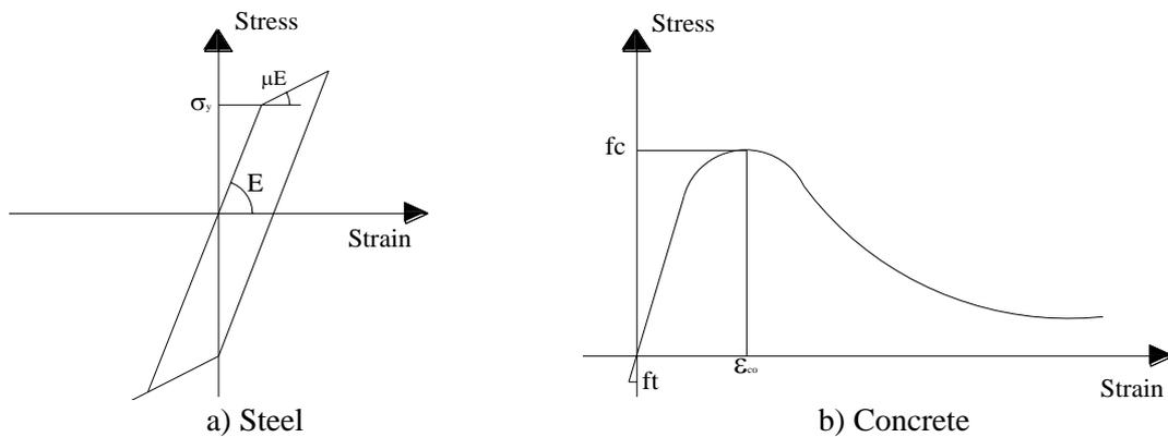
Fig. 2 Material models for steel and concrete
