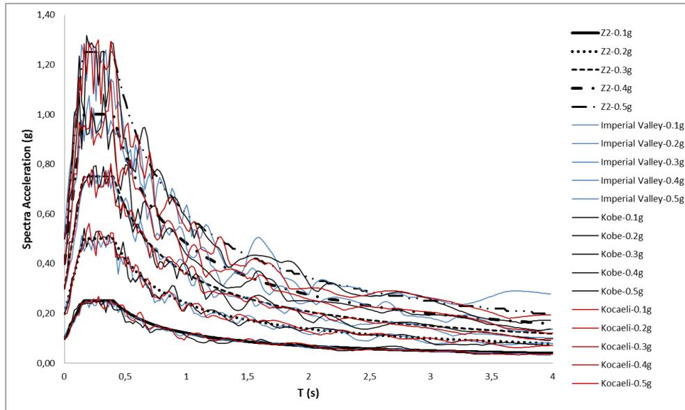
Fig. 3 Response spectra of the earthquake acceleration records scaled according to the elastic design spectrum for Z2 soil class and different ground accelerations
