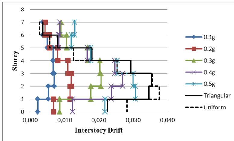
(a) Comparison of interstory drifts for scaled Imperial Valley earthquake and lateral static loads
