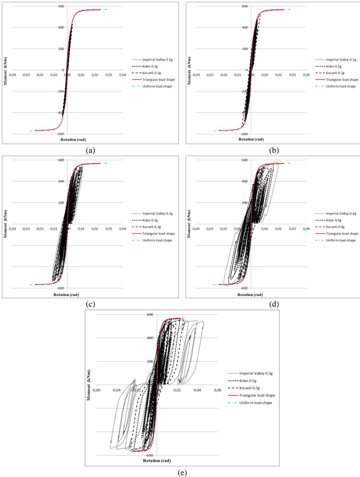
Fig. 9 Moment-rotation curves of lower end of C211a column under nonlinear static and dynamic loads
