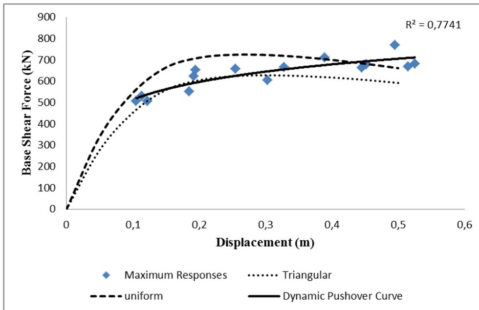
Fig. 6 Comparison of pushover curves obtained various load shapes and dynamic pushover curves
