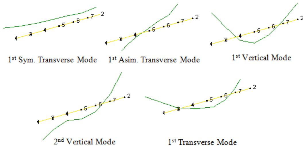
Fig. 16 The first five mode shapes obtained from the experimental measurements conducted on October 2010 (Case 3) by using SSI method
