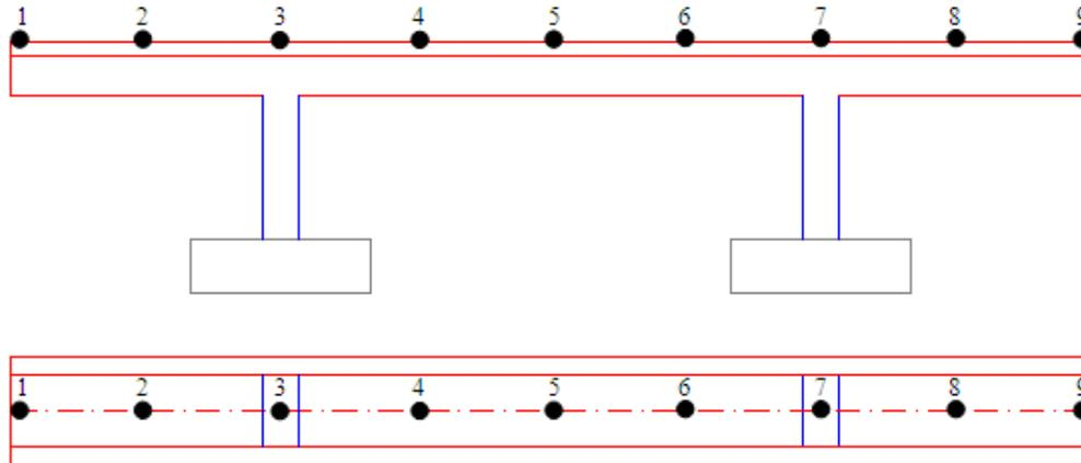
Fig. 7 Accelerometers locations on the bridge deck
