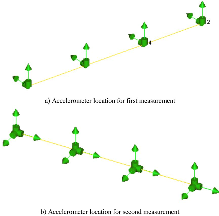
Fig. 17 Accelerometers locations on bridge deck for first and second test setups of Case 4
