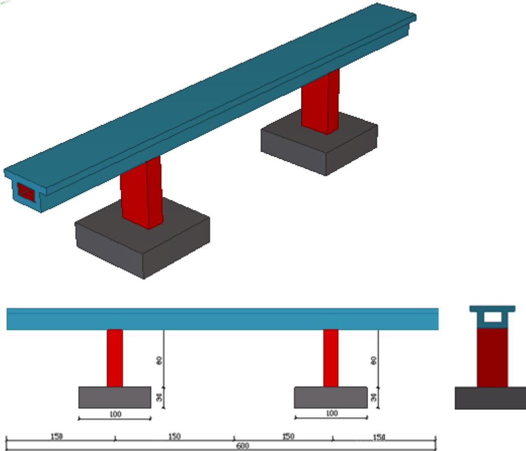
Fig. 1 Basic configuration of bridge model (all dimensions are in cm)
