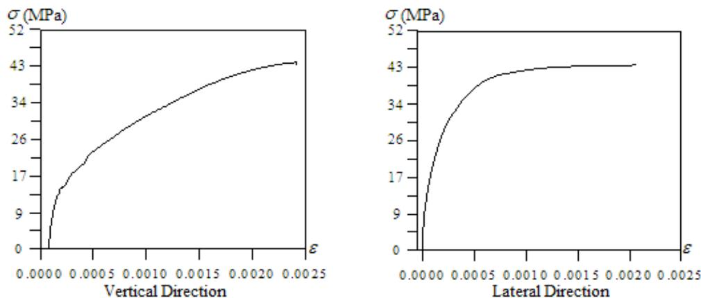
Fig. 5 The stress-strain diagrams attained from the sample compression tests
