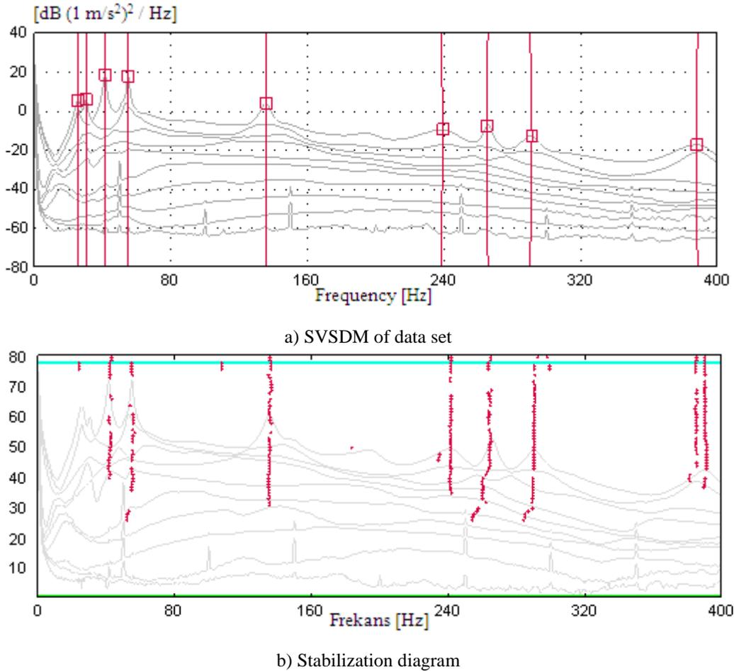
Fig. 9 SVSDM of data set and stabilization diagram of estimated state space models attained from the fifth test on June 2009 (Case 1)
