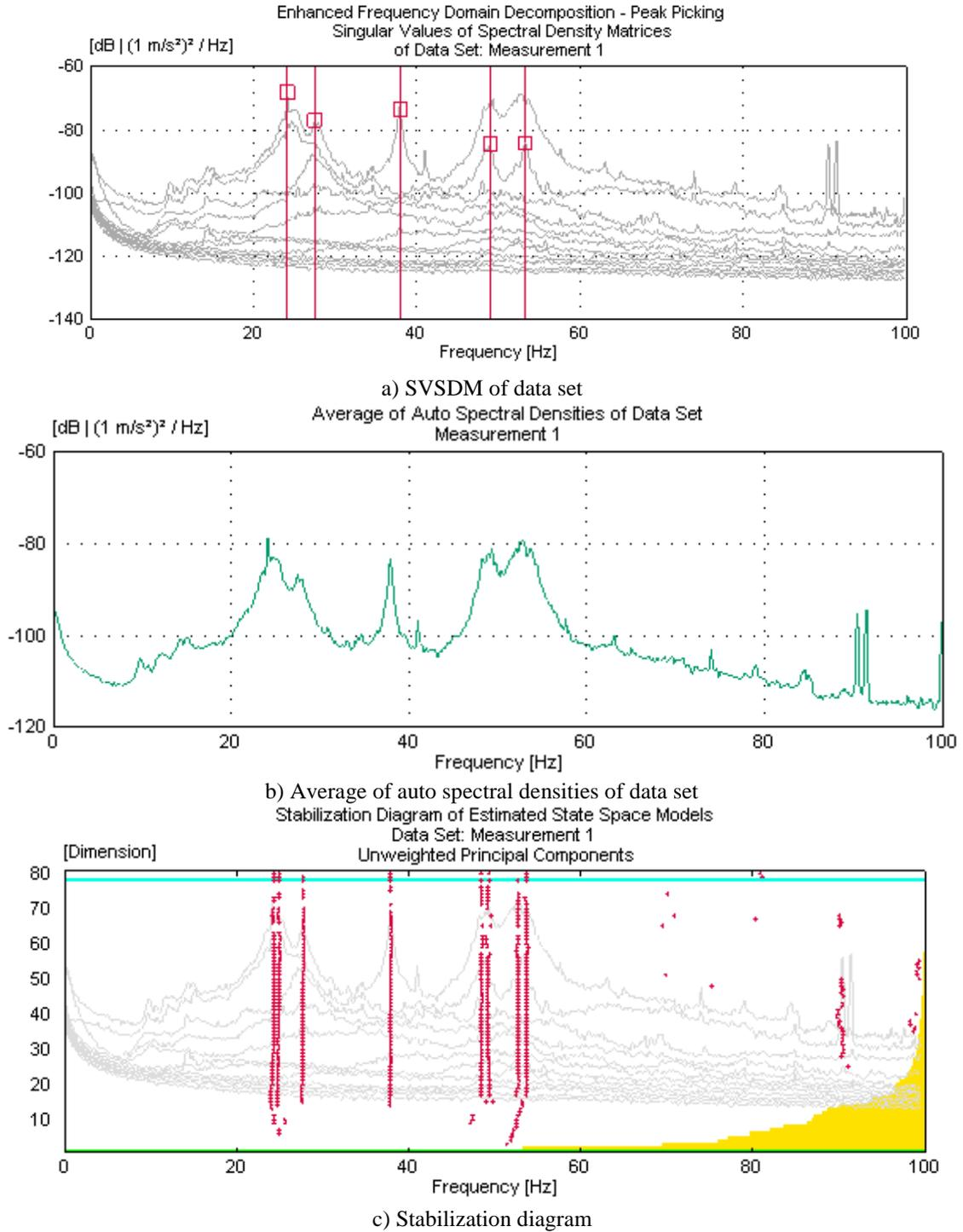
Fig. 19 SVSDM of data set, average of auto spectral densities of data set, stabilization diagram of estimated state space model and selected-linked modes across data sets attained from the second measurements using EFDD and SSI methods on February 2015 (Case 4)
