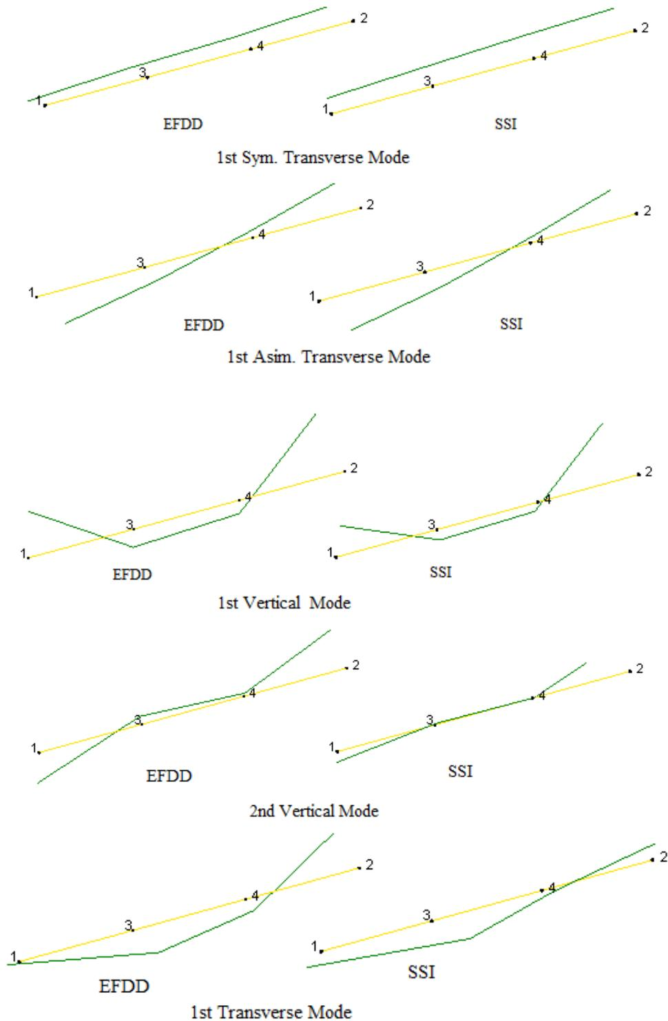
Fig. 20 The first five mode shapes obtained from the experimental measurements conducted on February 2015 (Case 4) by using EFDD and SSI methods
