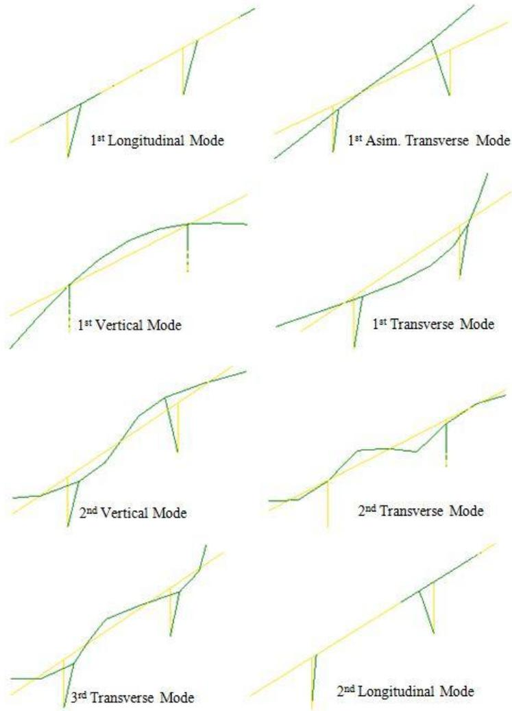
Fig. 10 The first eight mode shapes obtained from the experimental measurements conducted on June 2009 (Case 1) by using EFDD and SSI methods
