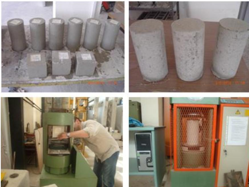
Fig. 4 Some view from the samples and compression tests
