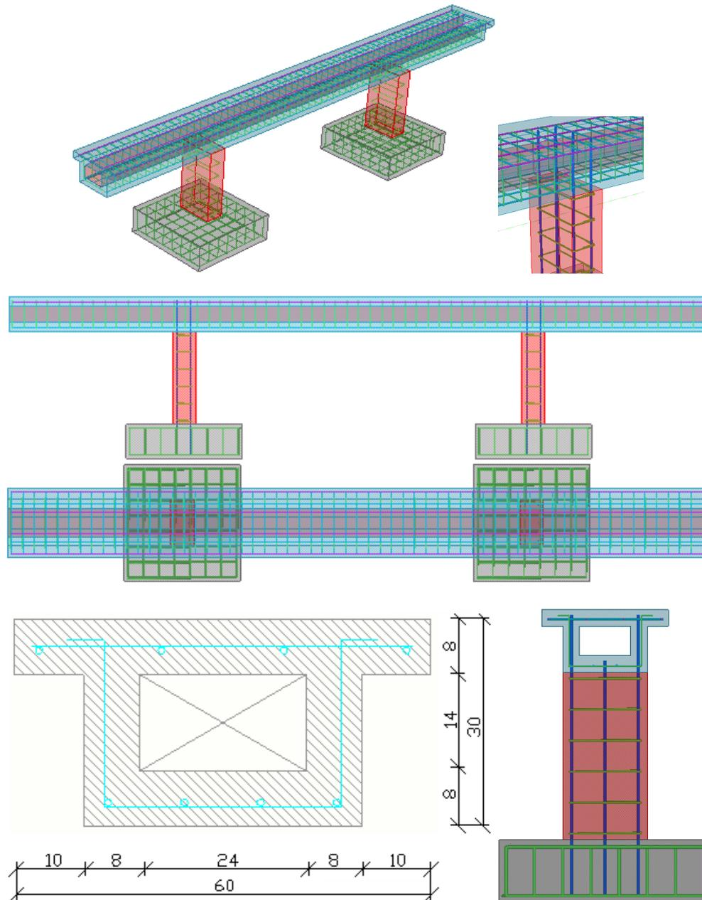
Fig. 2 Steel reinforcement details for each structural element (all dimensions are in cm)
