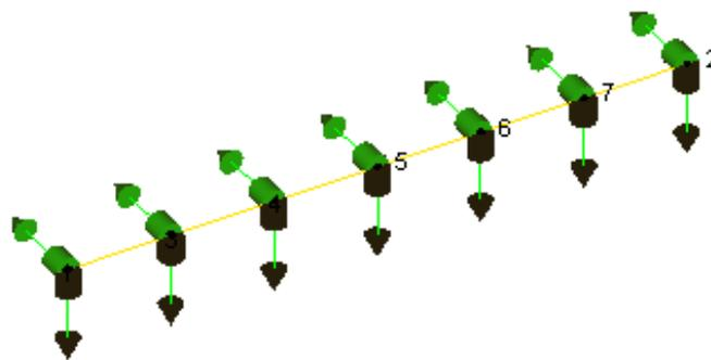
Fig. 11 Accelerometers locations on the bridge deck
