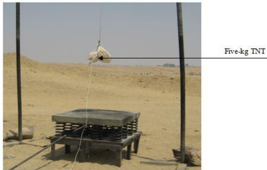
Fig. 18 Specimen No. 3 is subjected to five-Kg TNT at stand-off distance of 1m
