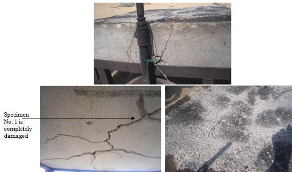
Fig. 15 Specimen No. 1 after subjecting to four-kg TNT explosive charge (Control RC panel without helical springs)
