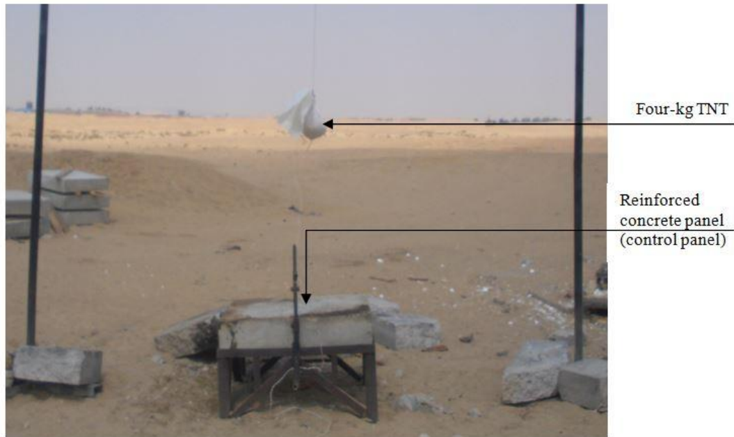
Fig. 14 Specimen No. 1 is subjected to four-kg TNT at stand-off distance of 1m (Control RC panel without helical springs)
