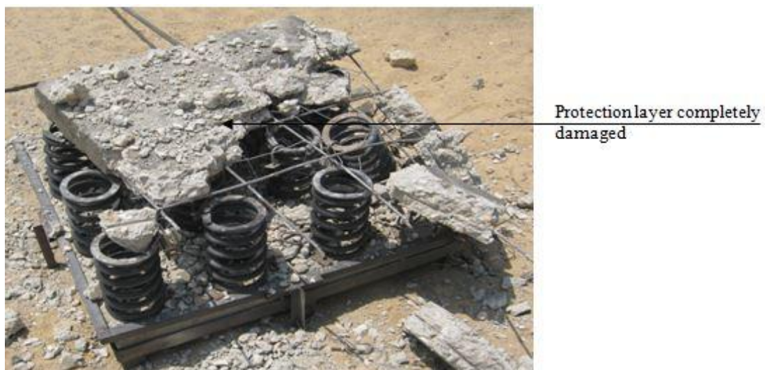
Fig. 21 Specimen No. 4 after subjecting to ten-kg TNT explosive charge
