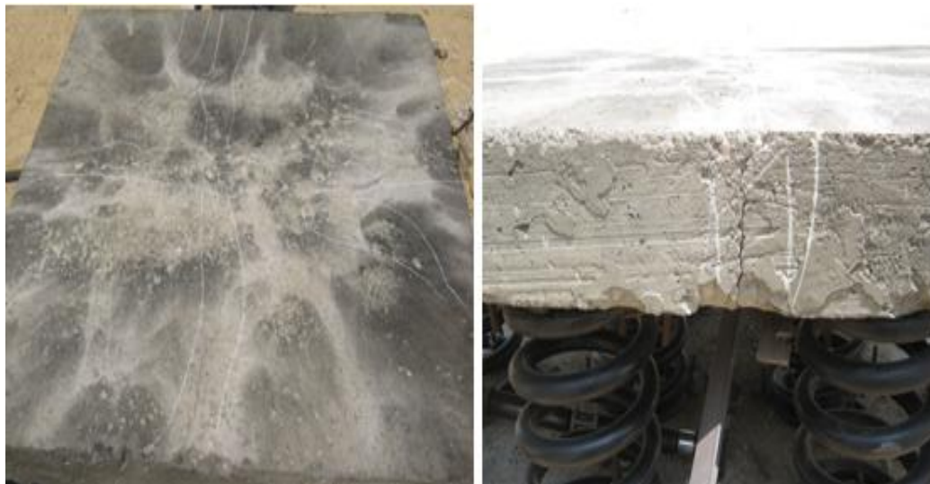
Fig. 19 Specimen No. 3 after subjecting to five-kg TNT explosive charge (Significant cracks appears through protection layer)
