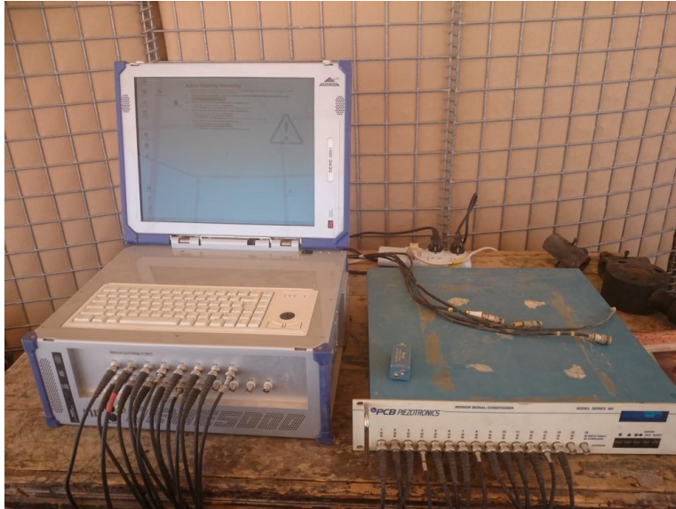
Fig. 4 Measurement instrumentation for field blast test
