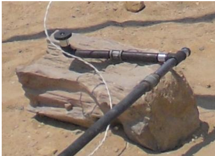
Fig. 5 Pressure sensor and cable protective system
