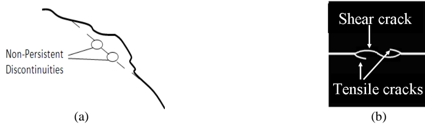
Fig. 1 (a) Rock bridges in discontinuously-jointed rock, (b) crack pattern in gypsum specimens in direct shear test
