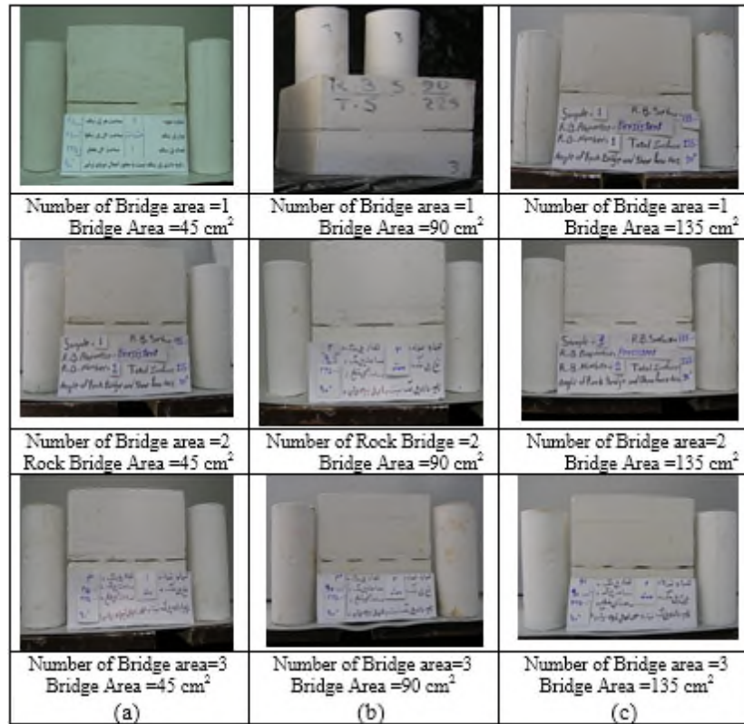
Fig. 4 The physical models consisting non-persistent joints
