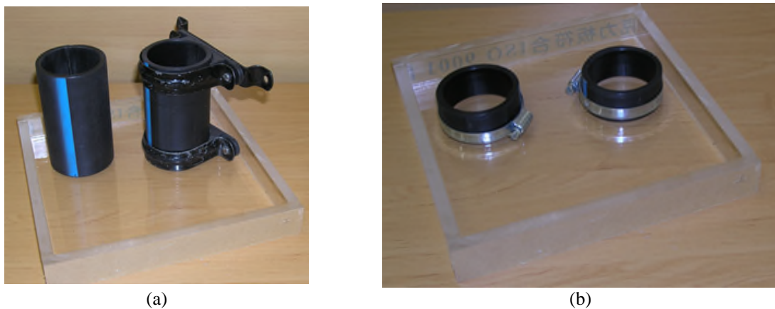
Fig. 2 (a) Cylindrical mold with 56 mm in diameter and 112 mm in length, (b) disc mold with 56 mm in diameter and 28 mm in thickness.
