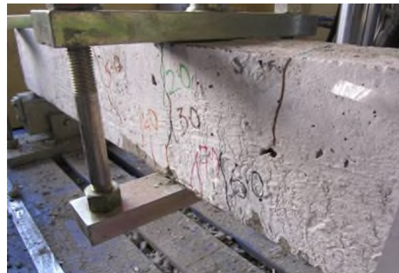
Fig. 4(b) Crack pattern on Reinforced SCC beam
