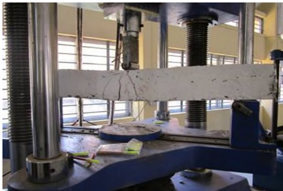
Fig. 4(a) Test setup of Reinforced SCC beam
