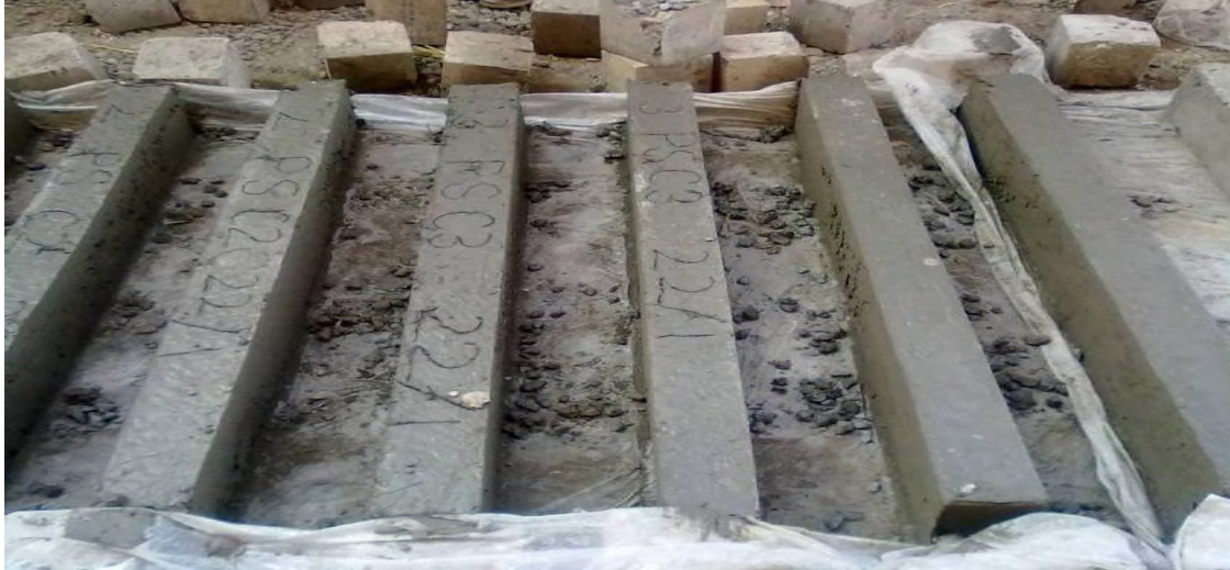
Fig. 2 Details of Cast flexural SCC members with different fiber dosages
