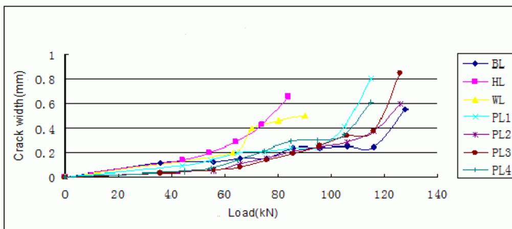
Fig. 6 Load-crack width curves of the tested beams
