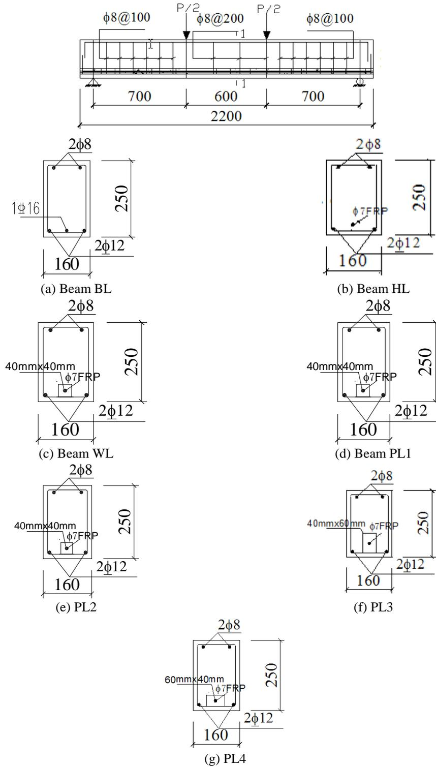
Fig. 2 Typical dimensions and geometry of tested beams
