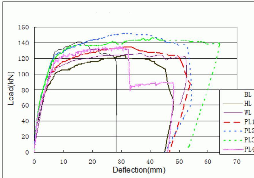
Fig. 5 Load-deflection curves of the tested beams
