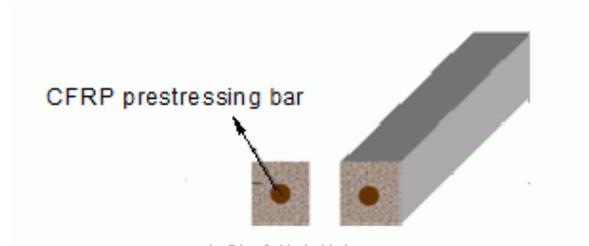
Fig. 1 Typical CFRP prestressed concrete prism(PCP)
