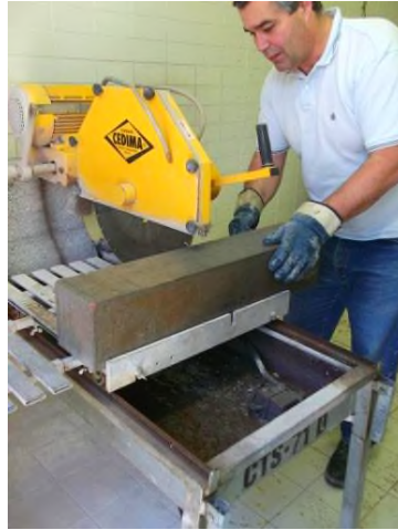
Fig. 1 Cutting the prismatic specimen
