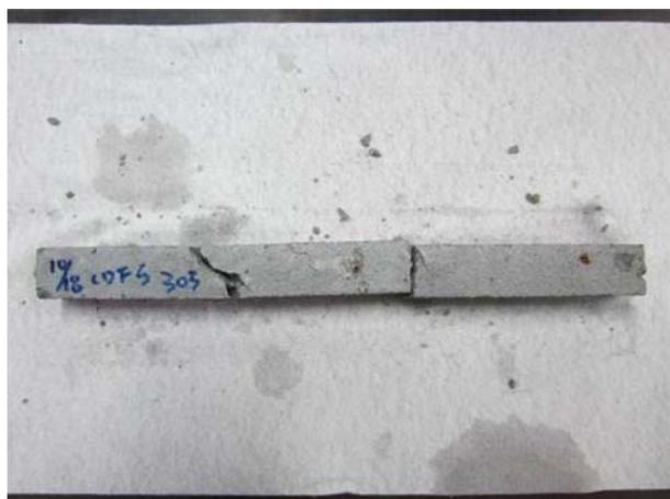
Fig. 4 The photo image of the sample with 30% DS (after the autoclave expansion)
