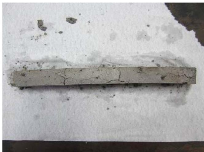
Fig. 3 The photo image of the sample with 20% BOF (after the autoclave expansion)
