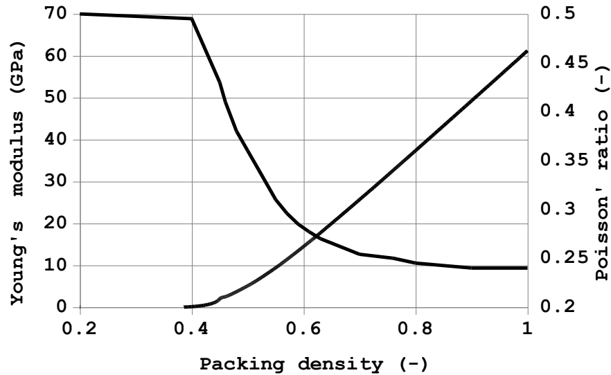
Fig. 11 Effect of packing density of C-S-H on its elastic properties calculated using SCS
